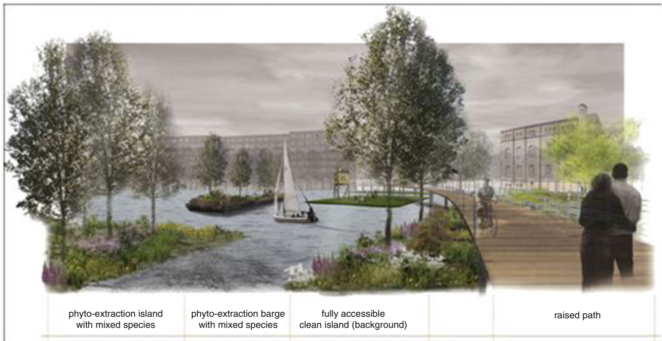
Fig. 5.7 Landscape typology “accumulation park.” This park is made accessible by a raised path and planted with a mixture of phytoextraction species combined with rows of poplars. From Theuws and Wilschut
