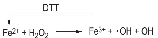
Fig. 20.1. The Fenton reaction.
