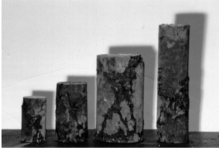
Figure 6. Mode of failure of cylinders of different sizes containing 2% by volume of hooked steel fibres
