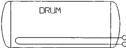
**FIGURE 8.12** Exchanger inside boiler drum.
