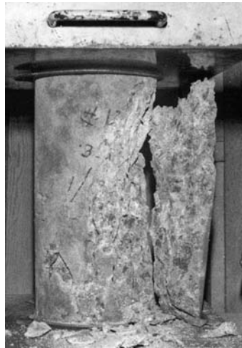
PHOTO 6.7 Failure patterns of higher strength concrete compressive test. (Photograph courtesy of E.G. Nawy et al.)
