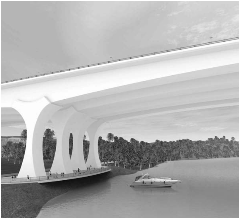
FIGURE 29.38 The pier shape creates a reflection of curved forms with continuous movement into the bridge superstructure (I-35W, St. Anthony Falls Bridge in Minnesota). Two main piers feature observation platforms along the edge of the river. The appearance underneath creates a visually clean and quiet space.
