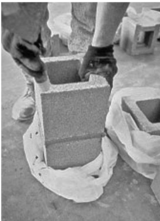
FIGURE 28.15 Masonry prism construction. (Courtesy of the National Concrete Masonry Association, Herndon, VA.)
