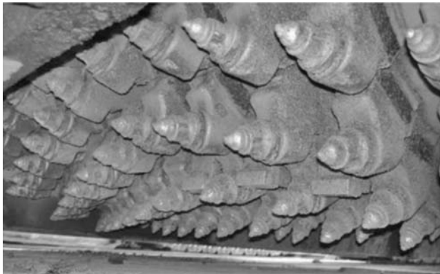
FIGURE 23.3 Fine milling heads spaced \leq 8 mm apart as shown are being used to minimize damage to the milled surface.
