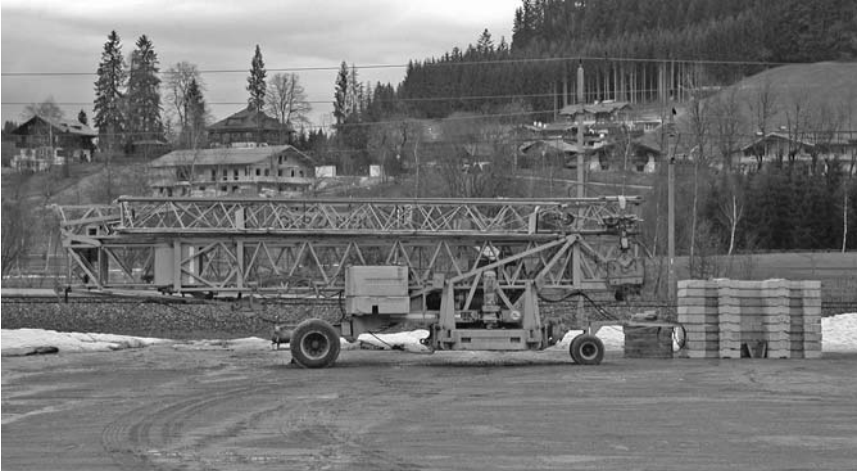
FIGURE 19.18 Bottom-slewing tower crane in towing position. Note the concrete ballast blocks, at the right of the picture, to be carried by the towing truck.
