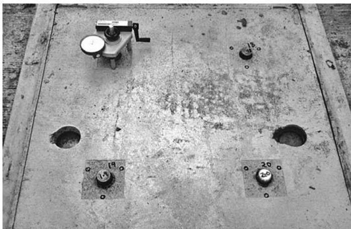
FIGURE 23.6 An overlay test patch is tested for bond strength.
