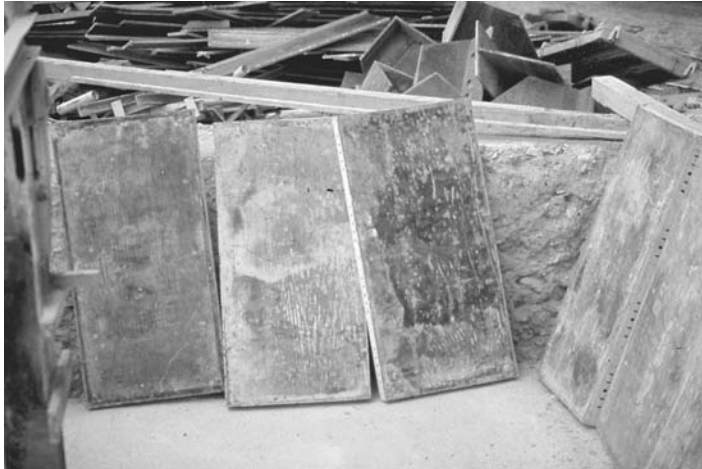
FIGURE 30.14 Poor-quality form surface where the dense plywood and its surface coating have been worn through repetitive usage.
