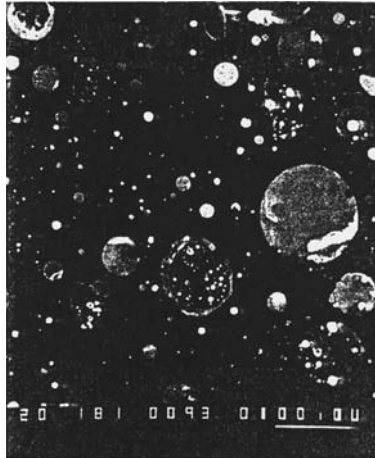
FIGURE 2.3 SEM micrograph of a lignite fly ash: backscattered electron image of a polished section of the dispersed sample. (From Malhotra, V.M. and Ramezaniapour, A.A., Fly Ash in Concrete , MSL 94-45(IR), Canada Center for Mineral and Energy Technology (CANMET), Ottawa, 1994.)
