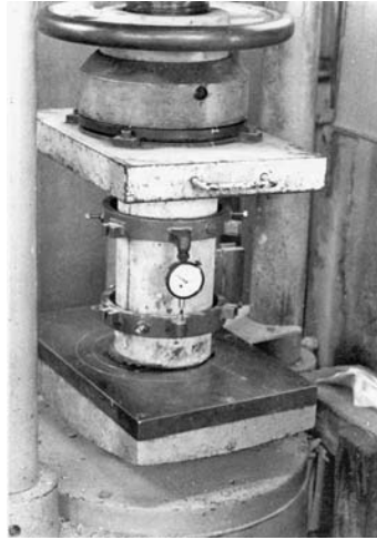
PHOTO 6.4 Cylinder compressive-strength testing set-up.
