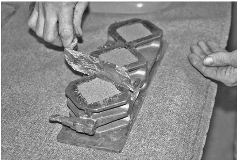
FIGURE 28.13 Masonry mortar cubes. (Courtesy of the National Concrete Masonry Association, Herndon, VA.)
