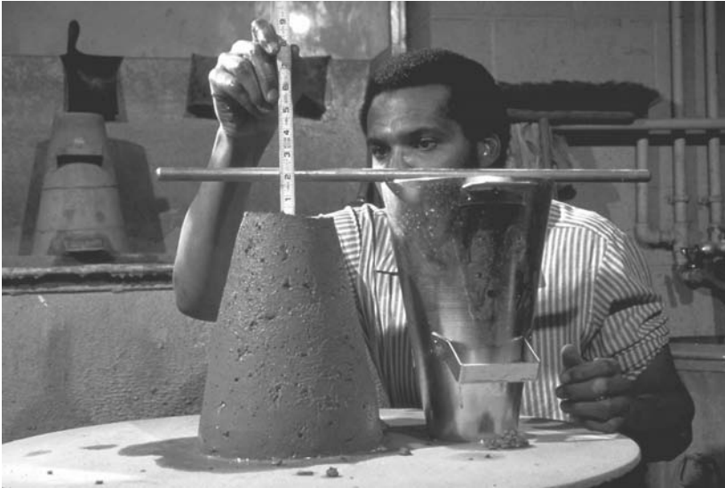
FIGURE 5.5 Consistency slump test of concrete. (Figure courtesy of the Portland Cement Association, Skokie, IL.)
