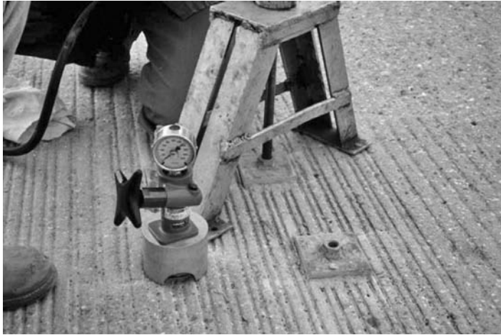
FIGURE 23.5 Metal disks or plates are bonded to the surface and pulled in tension.
