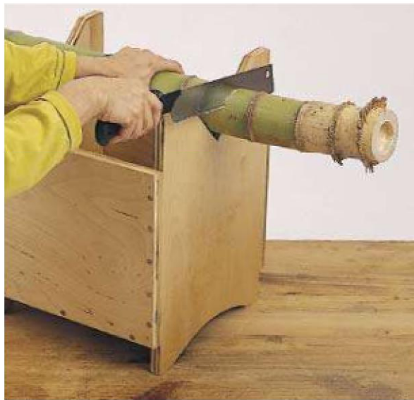
Photo 1: When using a Japanese cutting box, rotate the pole to get a clean cut.
