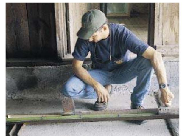
A worker at the Bamboo Farm, Savannah, Georgia, splits a pole through a blade welded onto an angle iron.
