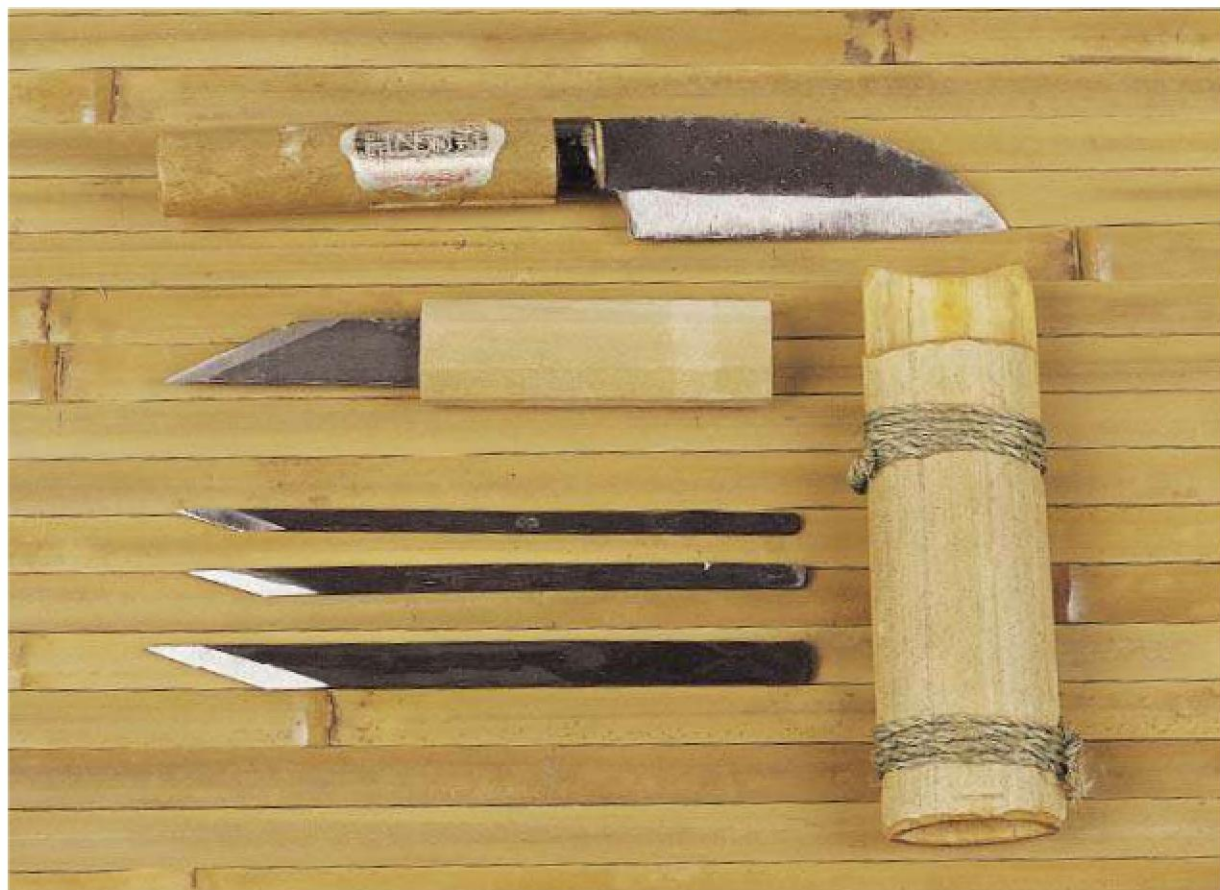
Japanese knives for splitting and cutting. KNIFE SHEATH ON RIGHT BY TAKEI AKINORI
