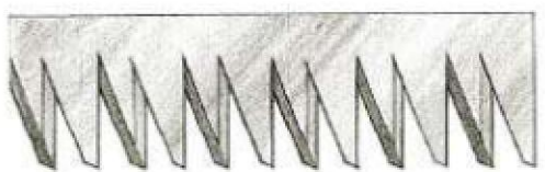
Japanese bamboo saws are “pull to cut,” cutting on the stroke moving toward your body.
