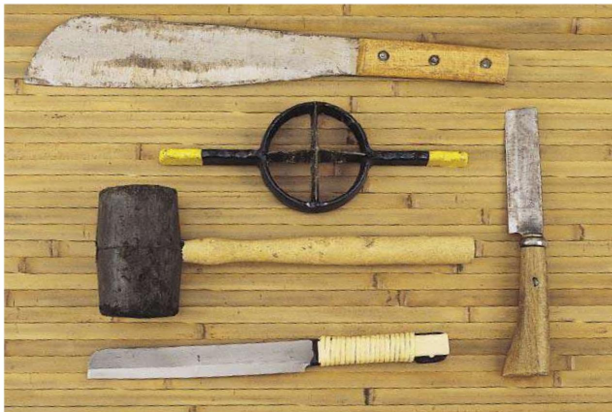
Clockwise from top: machete, splitting knife, take ware, rubber mallet, four-way splitter.
