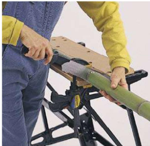
Photo 2: To eliminate “feathering,” hold the end of the bamboo while you cut.
