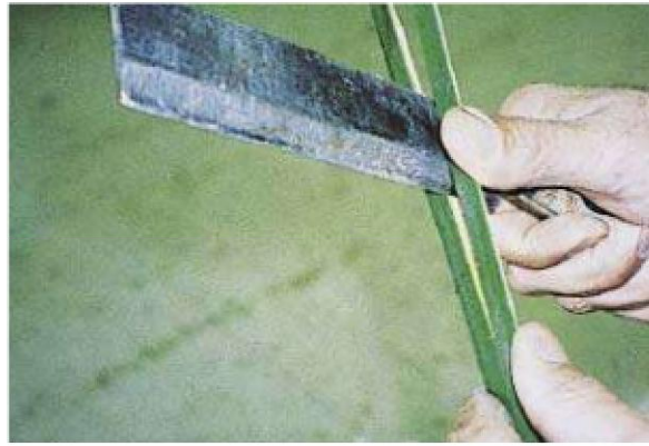
When splitting or removing the pith to make splints, wear leather work gloves until you've mastered the techniques. A blade that's sharp enough to cut bamboo can easily cut your fingers.
