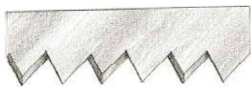
Western-style “push” saws such as hacksaws are primarily “push to cut,” meaning the teeth cut on the stroke moving away from your body.
