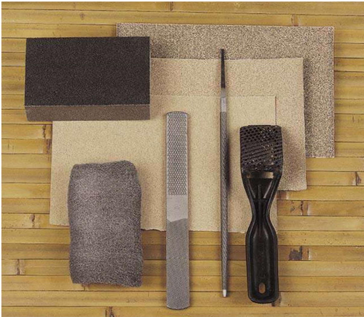
Materials and tools for sanding and smoothing. Left to right: sanding block, sandpaper, steel wool, flat rasp, round rasp, shaver.
