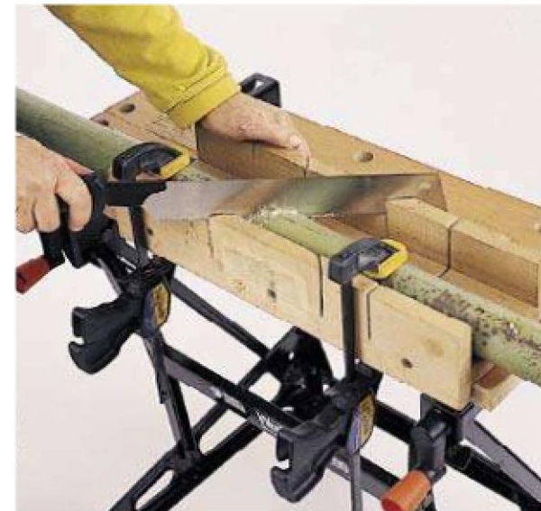
Photo 3: Using a miter box to cut bamboo at a 45- or 90-degree angle.
