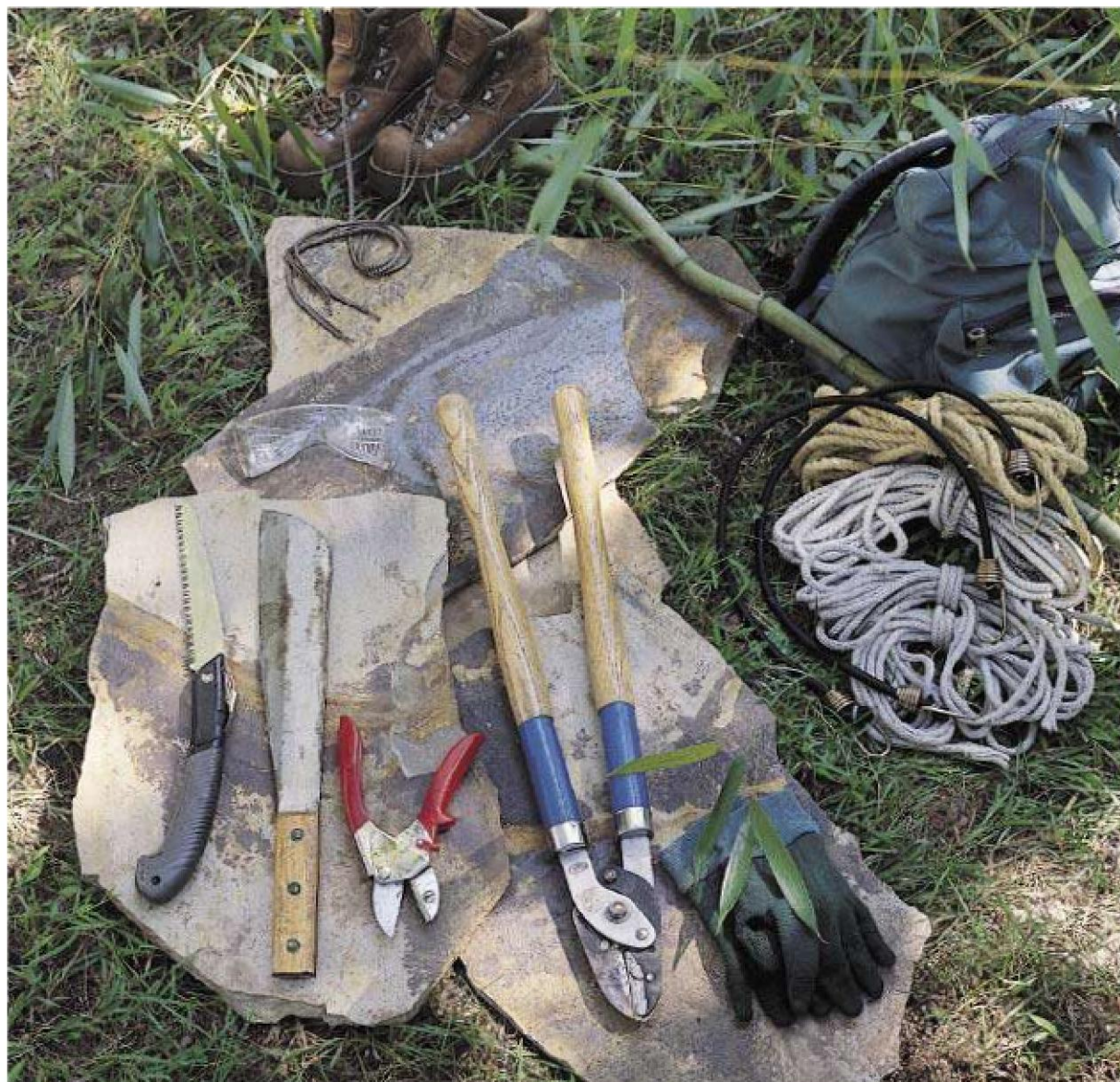
Harvesting tools include a collapsible tree pruning saw, machete or loppers, and hand pruners. Bring rope, bungee cords, collapsible sawhorses, and a tape measure, too.
