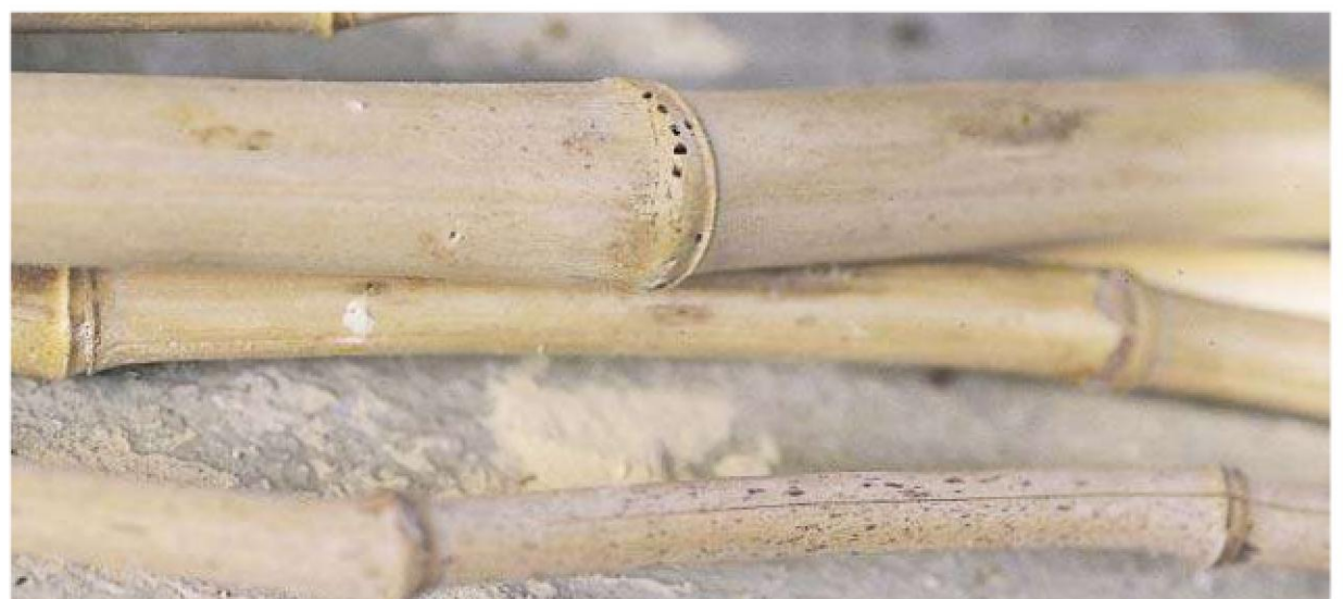
Pinprick-size holes in the bamboo and tiny mounds of finely ground powder are clues to insect infestation.
