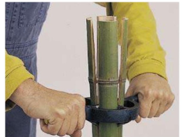
A four-way splitter makes splitting bamboo easy.
