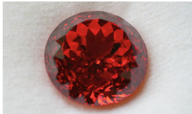
FIGURE 36.29. Single-crystal of rare earth (RE)-doped synthetic cubic zirconia that has been cut and polished.
