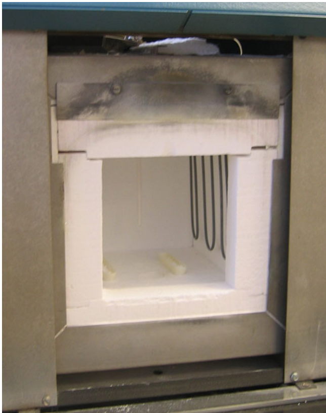
FIGURE 9.2. Small electrically heated box furnace.
