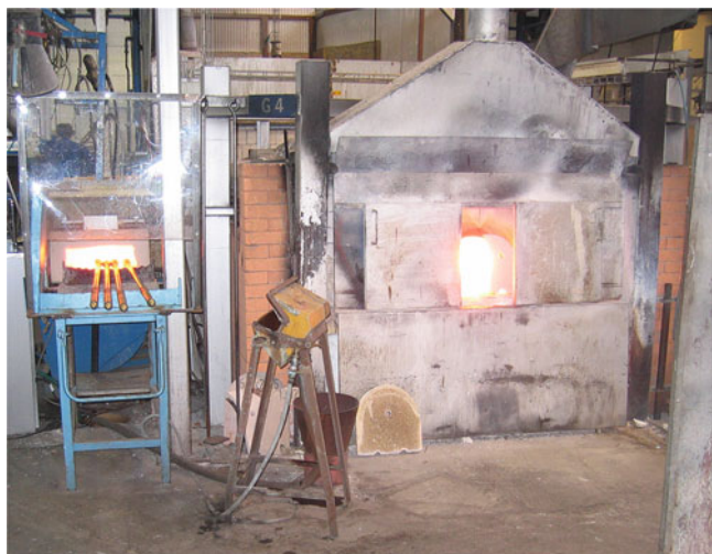
FIGURE 9.1. Gas-fired batch furnace used in a commercial glass-blowing operation.
