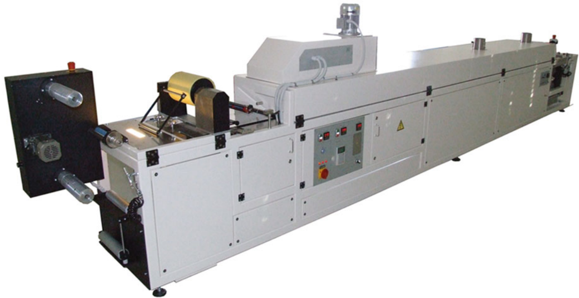
FIGURE 27.4. Example of an industrial tape casting machine.
