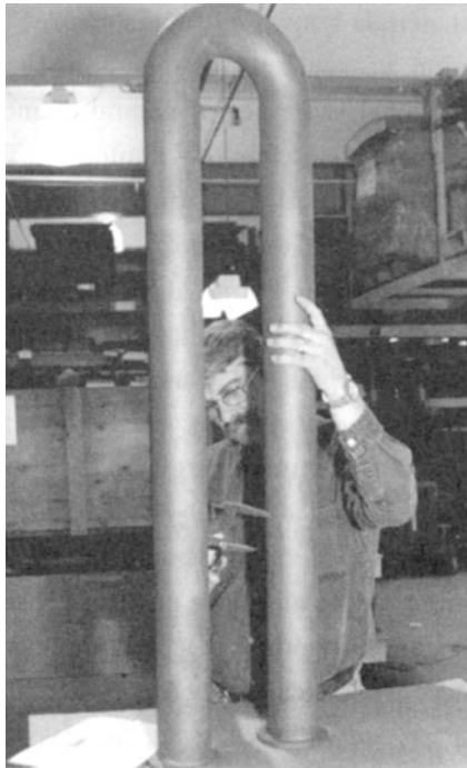
FIGURE 24.2. Radiant U tube produced by sintering SiC.
