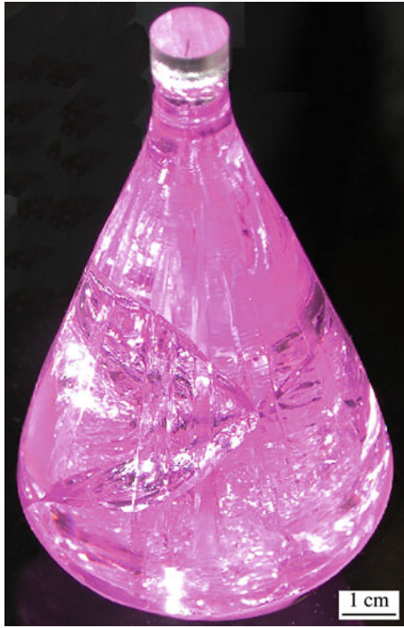
FIGURE 16.1. Cracking in an Nd-doped YAG boule.
