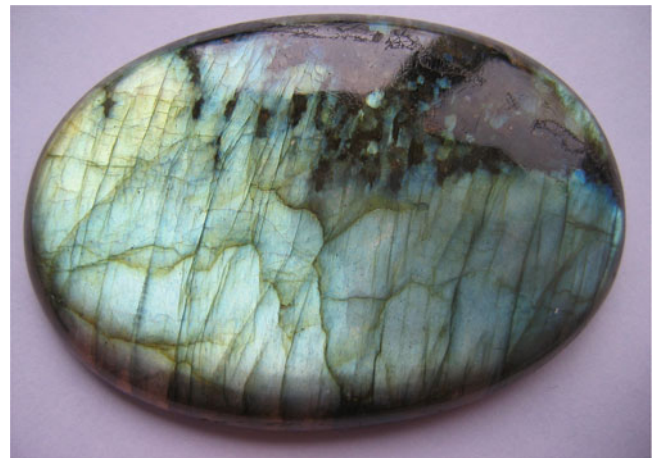
FIGURE 36.17. Laboradite causes an iridescence due to scattering by twin planes in the feldspar crystal.
