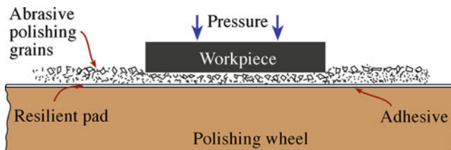
FIGURE 18.24. Polishing process using abrasive grains held in a soft pad. This method is the one most often used in university metallography laboratories.
