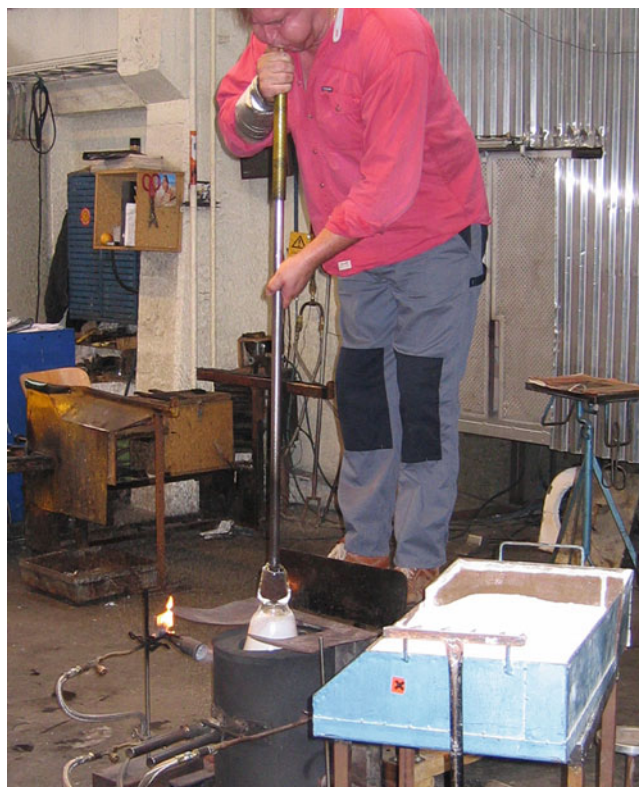
FIGURE 26.10. Blowing glass into a mold. (Note the worker’s bench, the annealing burners, and the box of frit.)
