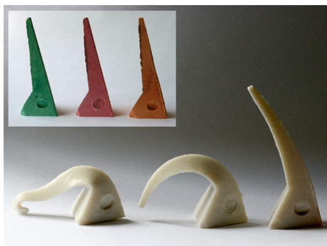
FIGURE 9.13. Orton cones: self-supporting type. The cones shown are 6 cm tall in their initial state.
