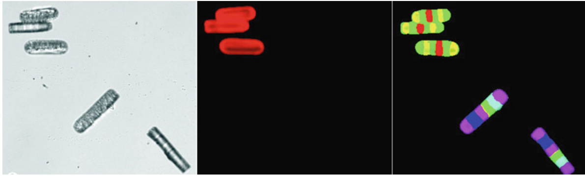
FIGURE 35.10. Microbarcodes from Corning. The cylindrical bars are typically 100 \mu\text{m} long and 20 \mu\text{m} in diameter.
