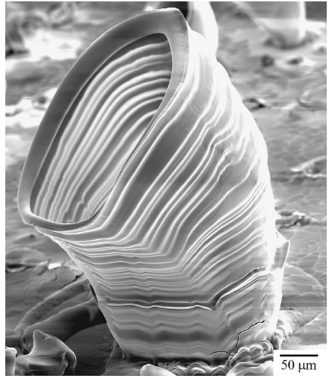
FIGURE 17.22. Microblown silica shape formed on oxidized SiC.
