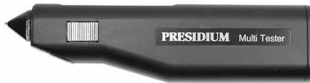
FIGURE 36.18. Pocket-size instrument for measuring thermal conductivity.
