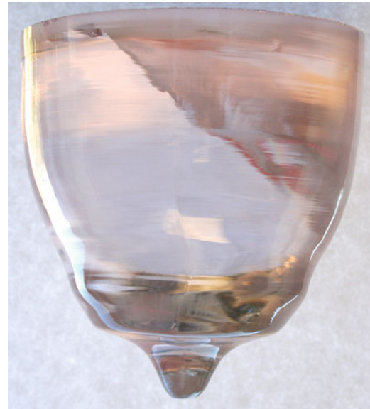
FIGURE 29.4. Sapphire boules grown by the Cz technique: 100–150 mm diameter, 300 mm long.
