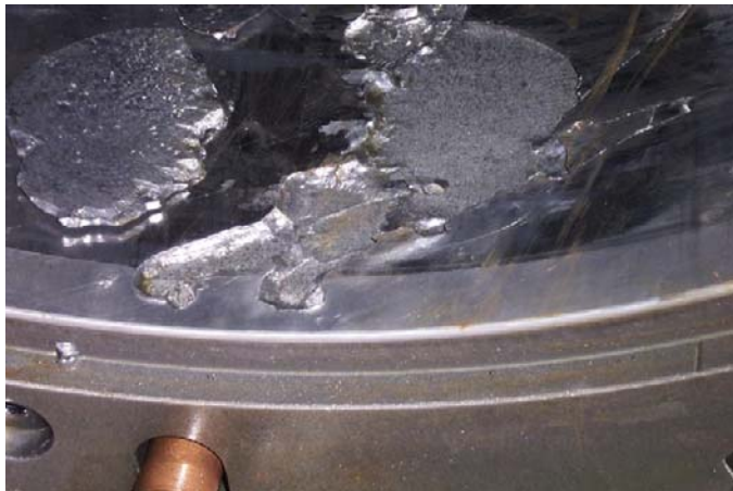
Propeller shaft white metal bearing
