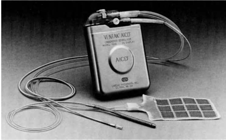
FIGURE 18.1. The automatic implantable cardioverter-defibrillator with, left to right, its bipolar right ventricular, superior vena cava, and apical patch electrodes.
