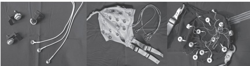
Figure 3.2 Electrodes and caps. Photograph of different types of electrodes and flexible caps, where electrodes are mounted and fixed according to the 10–20 system.
