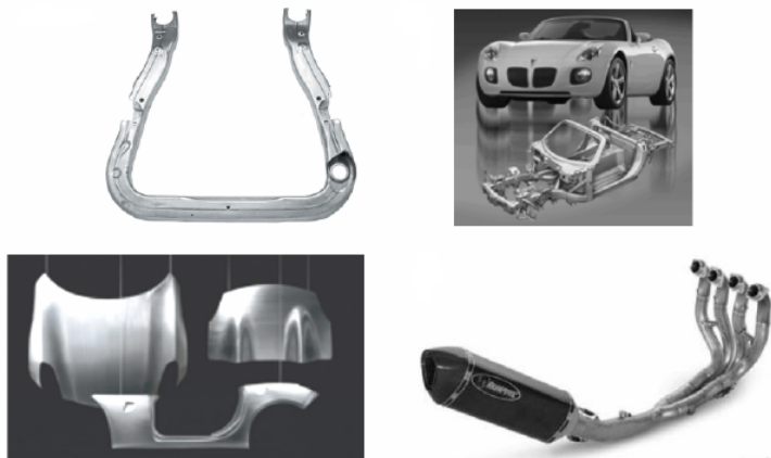
Figure 4.1. Examples of workpieces obtained by hydroforming [MAK 07]
