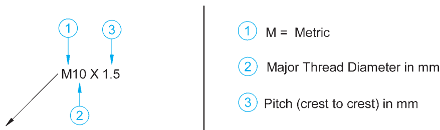
Figure 5-10 Typical Basic Metric Thread Specification
