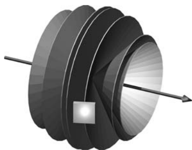
Figure 7.4 Schematic drawing of the first seven diffraction cones of Al at a wavelength of 1.64 Å. The box is at a detector position of 70^\circ for recording the (2 2 0) reflection.
