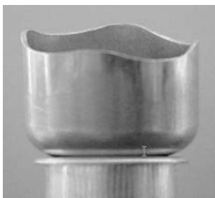
Figure 3.3 Al deep drawing cup showing the earring effect.
