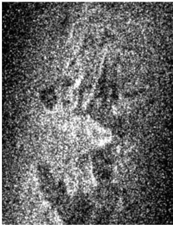
Figure 11.3 Exposure taken in the Fe (1 1 0) reflection from a perlitic steel rail. The peaks from ferrite and the white etching layer show a severe overlap. Due to several experimental parameters the exposures have been very noisy leading to noisy diffractograms for the individual pixels.
