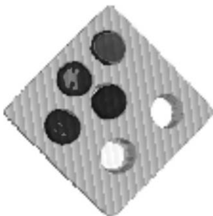
Figure 15.27 Reconstruction of an aluminum box having six holes, four were filled with different weight percentages (wt.%) of D_2O and \beta -carotene (see also Figure 15.26).
