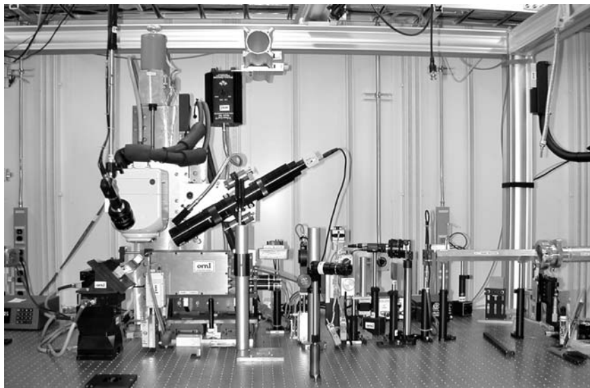
Figure 20.8 The 3D X-ray crystal microscope on beamline 34-ID-E. The components are mounted on an optical table, which allows new optical approaches to be rapidly tested.
