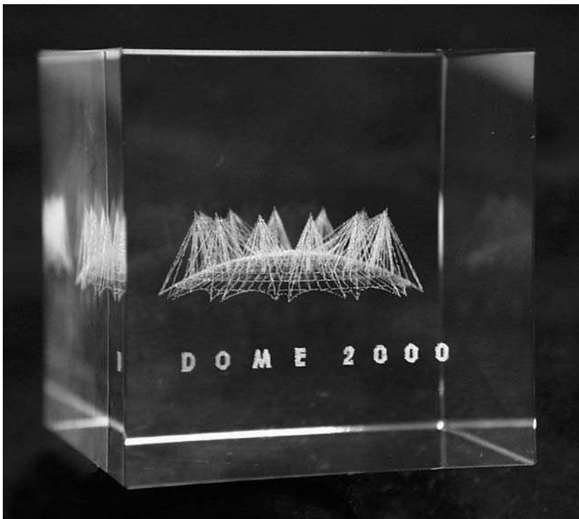
Figure 10.2 Three-dimensional image made by controlled laser microcracking in acrylic
