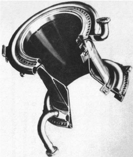
Figure 11.8 Main combustion chamber liner for space shuttle main engine, which is laser remelted to improve mechanical properties. (Source: Biliyar Bhat, NASA Marshall Space Flight Center, Huntsville, AL, USA)
