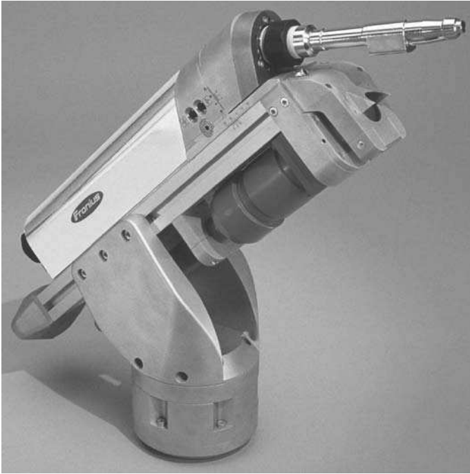
Figure 16.11 Hybrid Nd:YAG laser–MIG welding head. (Source: Herbert Staufer, Fronius, Wels-Thalheim, Austria)
