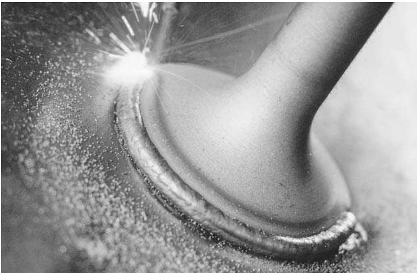
Figure 12.1 CO 2 laser beam cladding of a valve rim with cobalt-based hardfacing powder. (Source: Tero Kallio, Lappeenranta University of Technology, Finland)
