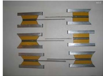
In accordance with the theoretical recommendations the second type of specimens were made so, that the opening angle of composite material equal  $70^\circ$  and  $50^\circ$  and opening angle of metal base equal  $180^\circ$ .
