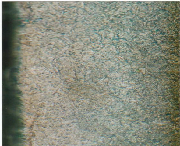
Figure 3. Microstructure of the local bolt sample before nitrocarburization (magnification 500x)
