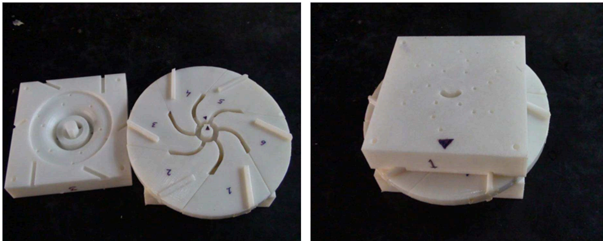
(i) Exploded view of Impeller mould (ii) Assembled view of Impeller mould
