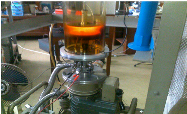
Figure 1: The radio-frequency plasma nitrocarburizing apparatus for this experiment
