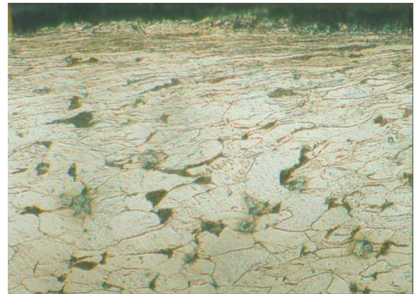
Figure 6. Microstructure of the local bolt sample after nitrocarburization at a temperature of 400°C for 5 hours (magnification 500x)
