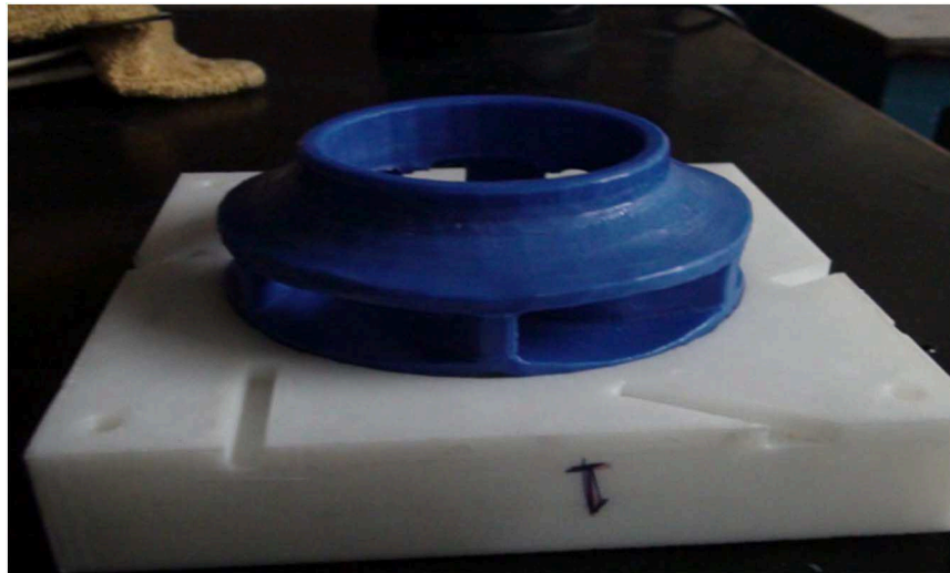
(i) Wax pattern of impeller in the mould
