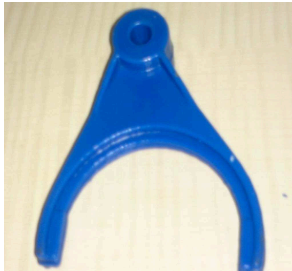
Fig.8 Wax pattern produced through from the chemically treated fork mould
