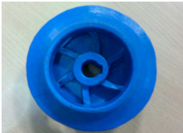
(ii) Top view of wax pattern of impeller
