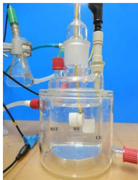
Fig. 1 Corrosion cell set up.
