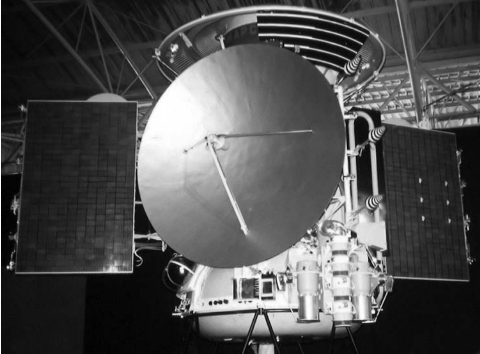
A mockup of the Soviet Mars-71P spacecraft. The conical heat shield of the lander is at the top. The black and white striped object is the lander's thermal radiator for the interplanetary cruise. (Courtesy Patrick Roger-Ravily)
