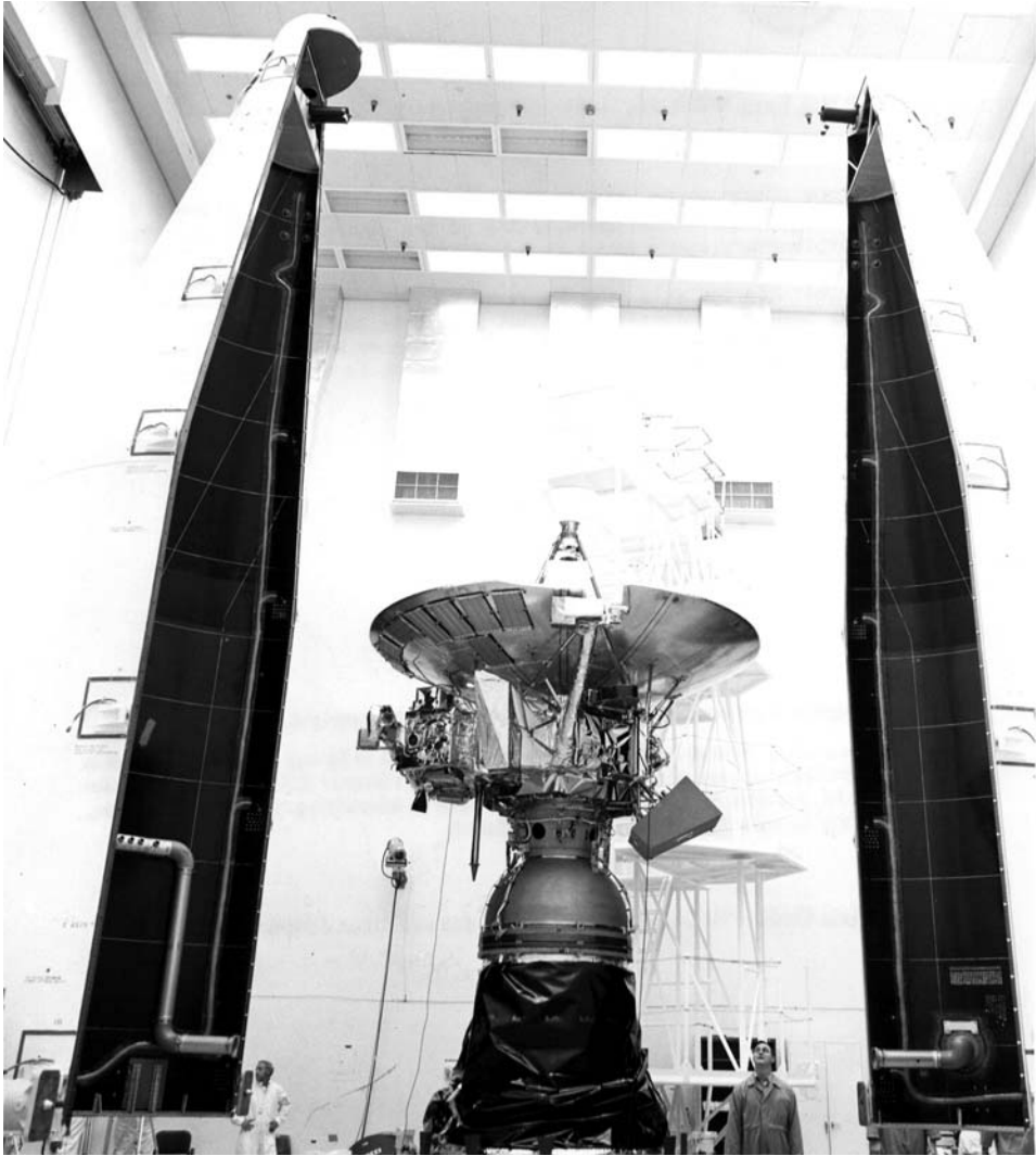
Pioneer 10 about to be enclosed by the aerodynamic shroud of its launch vehicle. The trapezoidal object protruding from the spacecraft to the right is the pod containing the 'Sisyphus' meteoroid-asteroid detector.
