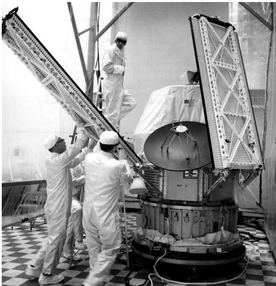
The ill-fated Mariner 8 spacecraft is prepared for launch. The high-gain antenna and the small horn antenna for communications during Mars orbit insertion are visible.
