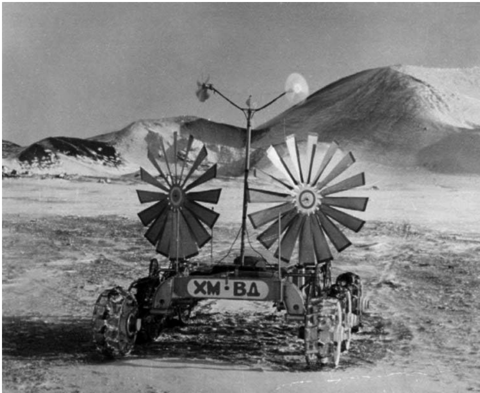
The wind-driven KhM-VD rover prototype designed for use on Venus. (Courtesy of VNII-TransMash)
