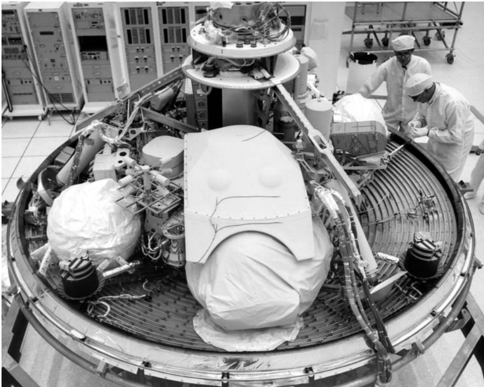
Preparing the Viking 2 lander. It is mounted inside the forward heat shield and the technicians are standing directly in 'front' of the two cameras (the white cylinders mounted on top of the craft).
