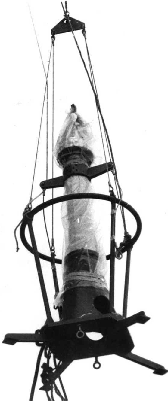
Pioneer 4 and the upper stage of its launch vehicle being hoisted to the Juno rocket. This spacecraft would become the second to venture in solar orbit, and the first US-made.
