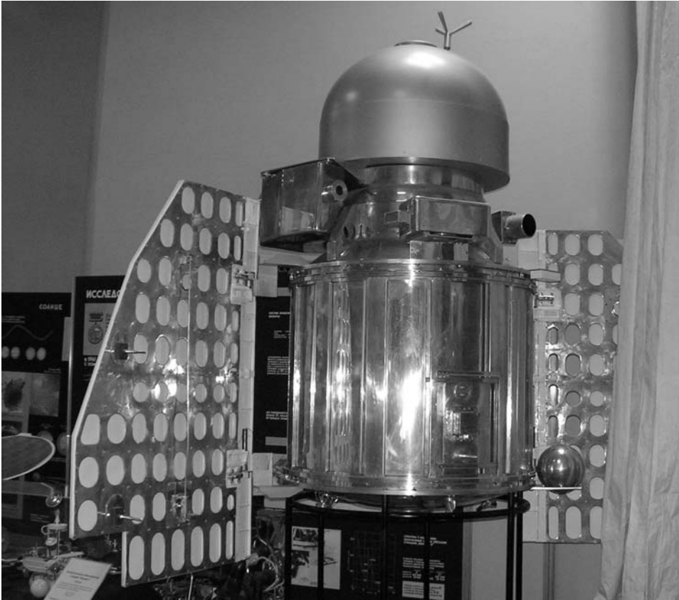
A model of Venera 1. This is the Earth-facing side of the spacecraft, but the high-gain antenna is not mounted. (Courtesy of Basil Pivovarov)
