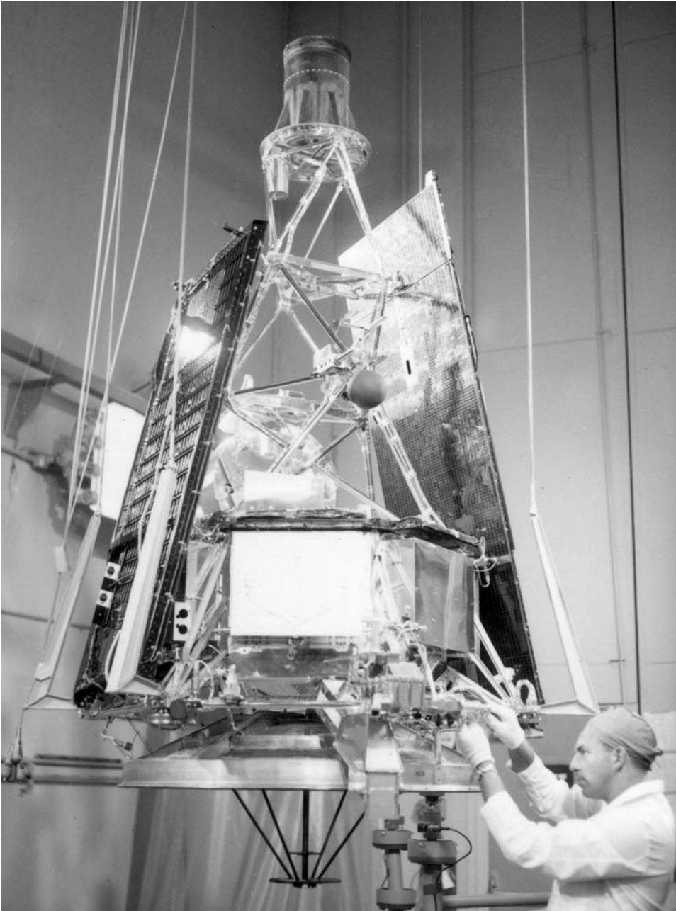
A Mariner R spacecraft being prepared for launch. The parabolic antenna is folded beneath the bus, and several scientific instruments can be seen. The radiometers are on the opposite side of the spacecraft. (Courtesy of NASA/JPL/Caltech)
