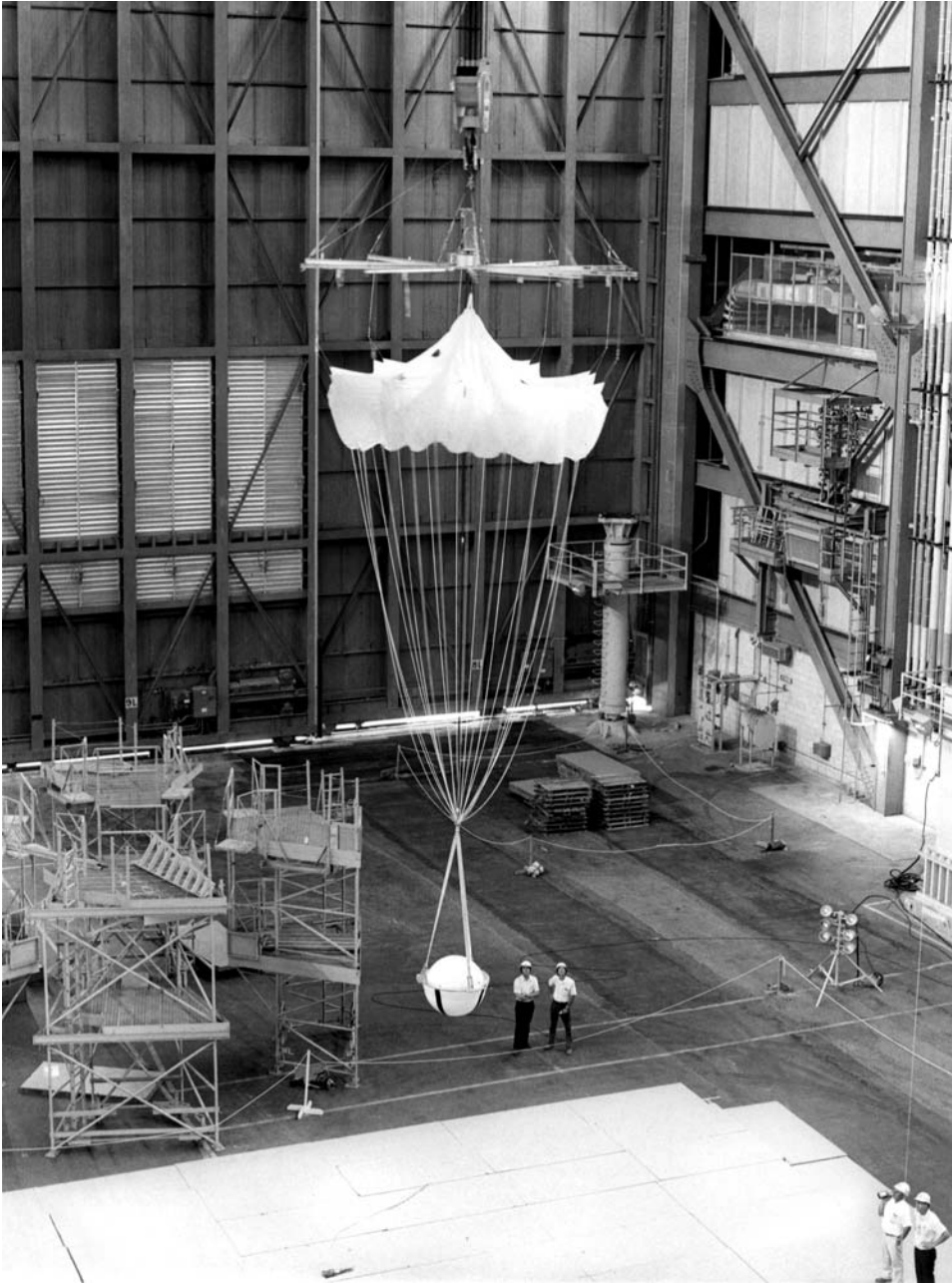
To test the parachute system of the Pioneer Venus large probe, models were released inside one of the largest enclosed structures on Earth, the Vehicle Assembly Building at the Kennedy Space Center.
