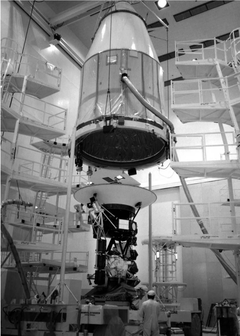
Lowering the aerodynamic shroud of the launch vehicle over Voyager 2. The circular disk on a side of the bus is the 'Sounds of Earth' recording.
