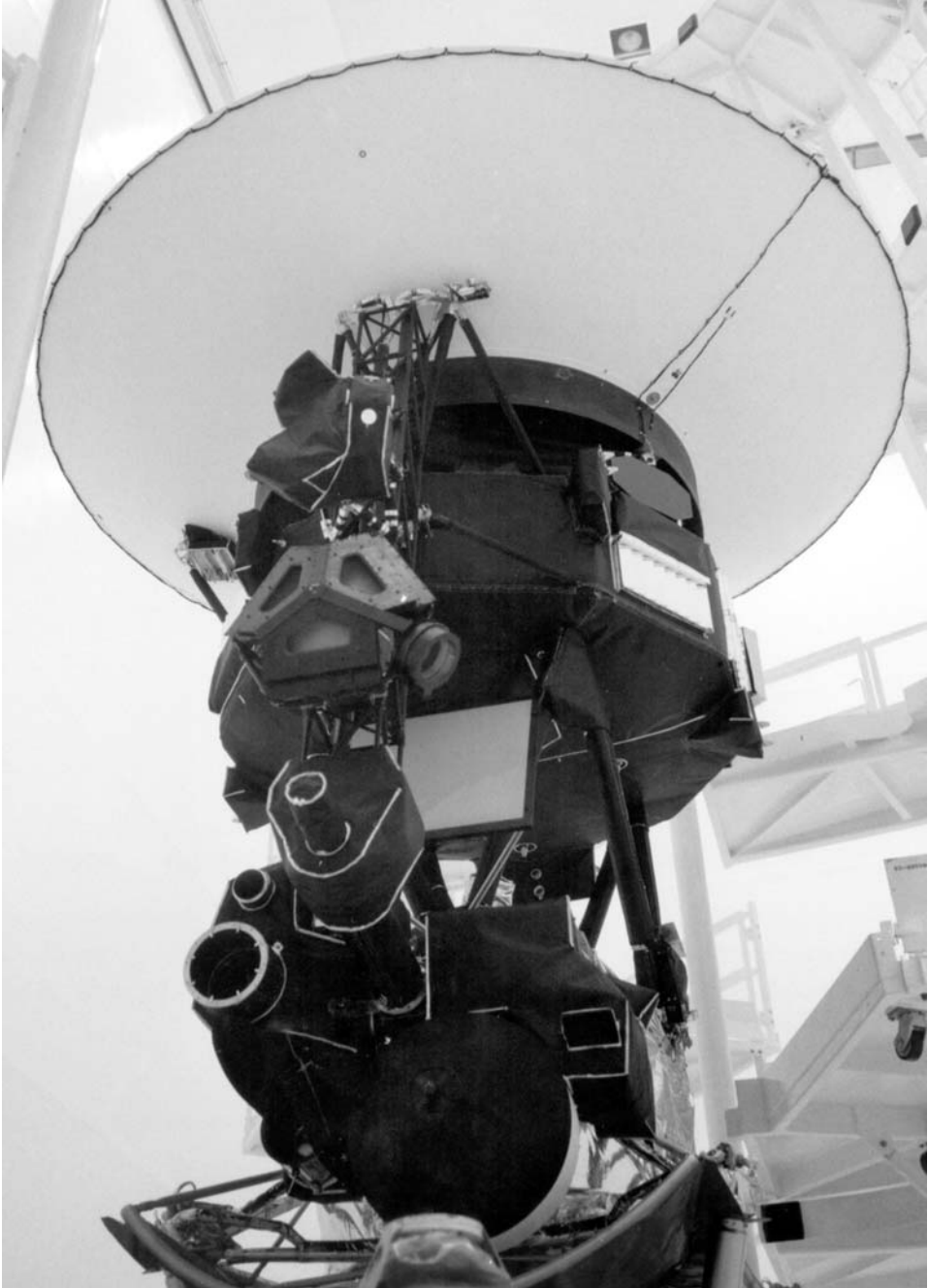
Preparing a Voyager spacecraft for launch. Note that the scan platform is in its most compact configuration with covers protecting its optics. (Courtesy of NASA/KSC)
