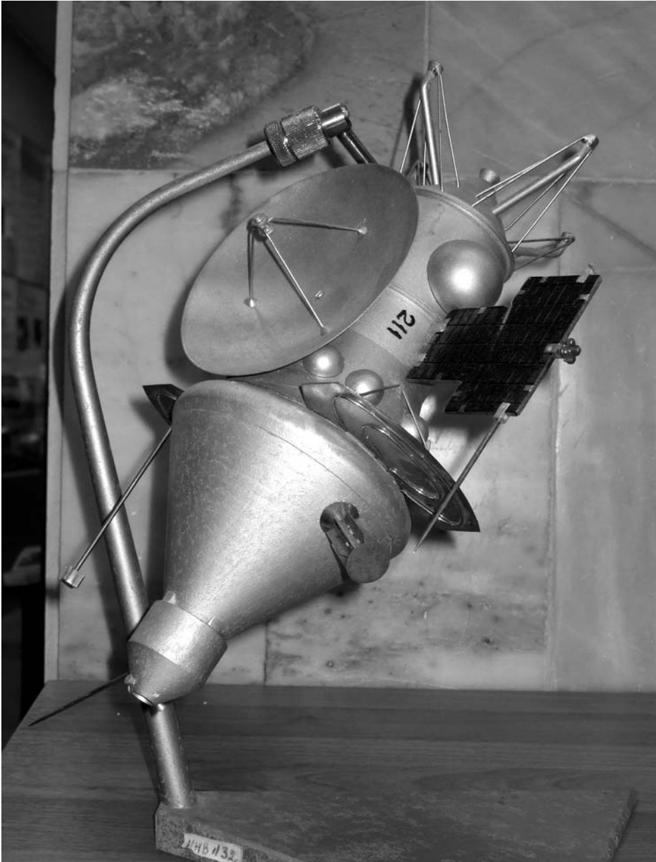
This is said to be a promotional model of a possible configuration for a Soviet probe for Mercury under study at TsNIIMash that would be powered by a combination of solar panels and RTGs, but other sources describe it as a Jupiter probe. (Courtesy of the TsNIIMash museum)
