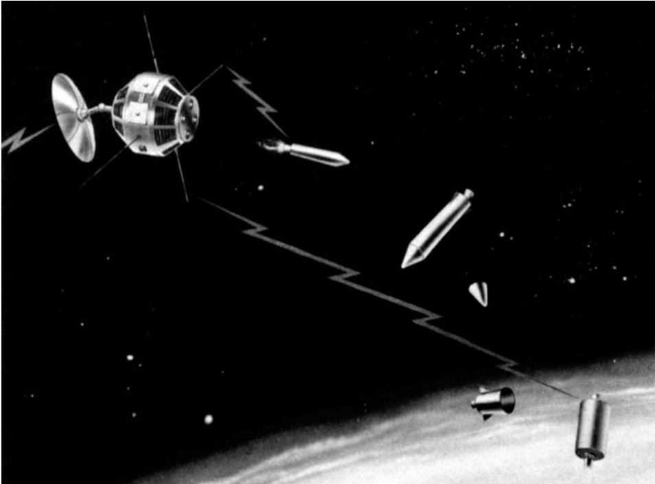
An early NASA Marshall Space Flight Center proposal for a Venus entry probe that would be delivered by a flyby bus.
