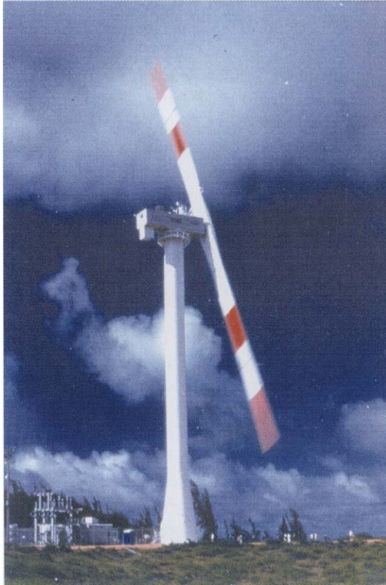
FIGURE 9.20 Obstruction markings. Painted with alternating bands of red and white. Hawaii. (Courtesy Paul Gipe.)
