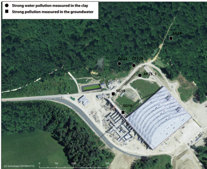
Fig. 7.2 Impacts of the Bonfol landfill on the nearby groundwater as measured in 2001 (Satellite image of the site (2007) reproduced by permission of Swisstopo (DV084371). Data from (CSD Ingénieurs et Géologues SA & Mireco, 2001). Please note that the image shows the site as it is now, notably with an excavation hall which did not exist in 1994. For a picture that better reflects the state of the site around this time please consult (CSD Ingénieurs et Géologues SA & Mireco, 2002))
