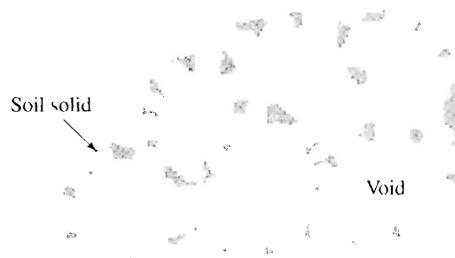
**Figure 3.23** Honeycombed structure
