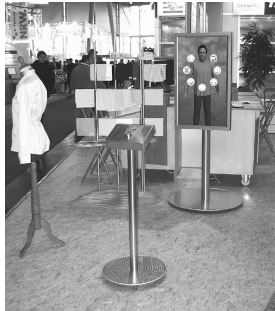
Fig. 4: System prototype at the CeBIT 2006 fair, Hanover, Germany; knob and buttons device (in the middle) and 3D product visualization with superimposed GUI showing the top menu level (right)
