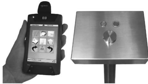
Fig. 3: PDA (3D interaction mask) and knob and buttons device
