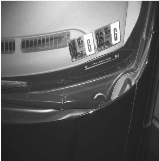
Figure 2: The vehicle identification number on the dash board below the front windscreen
