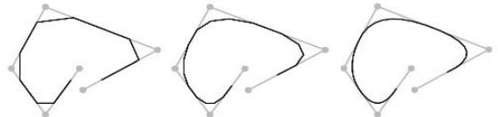
Fig. 3. Chaikin's algorithm applied to a control polyline three times, subsequently from left to right.
