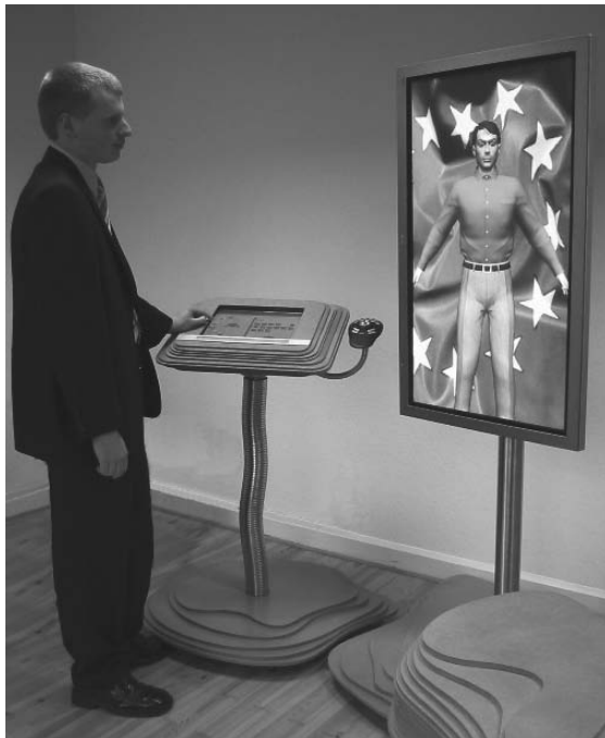
Fig. 2: Virtual Reality prototype with touch screen (left), ShuttlePRO device (attached right hand of the touch screen) and 3D scene display (right)
