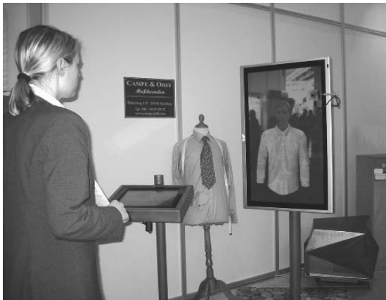
Fig. 1: Augmented Reality prototype with touch screen (left), large display (right) with video camera on right edge and test person with symbol card
