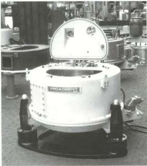
Figure 7.12 900 mm diameter simple manual discharge centrifuge (Broadbent Centrifuges)
