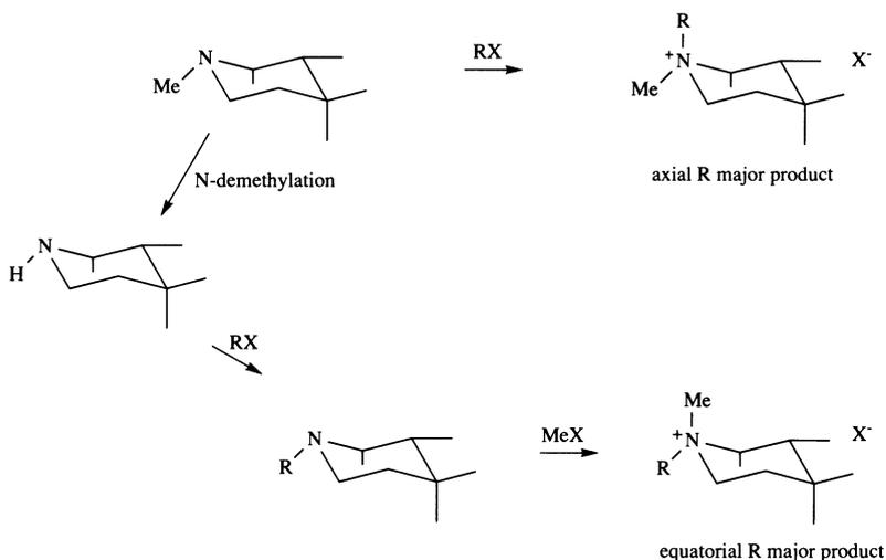
**Scheme 13.3.** Preparation of diastereoisomeric quaternary salts of opiates (partial structures shown centered around ring D).
