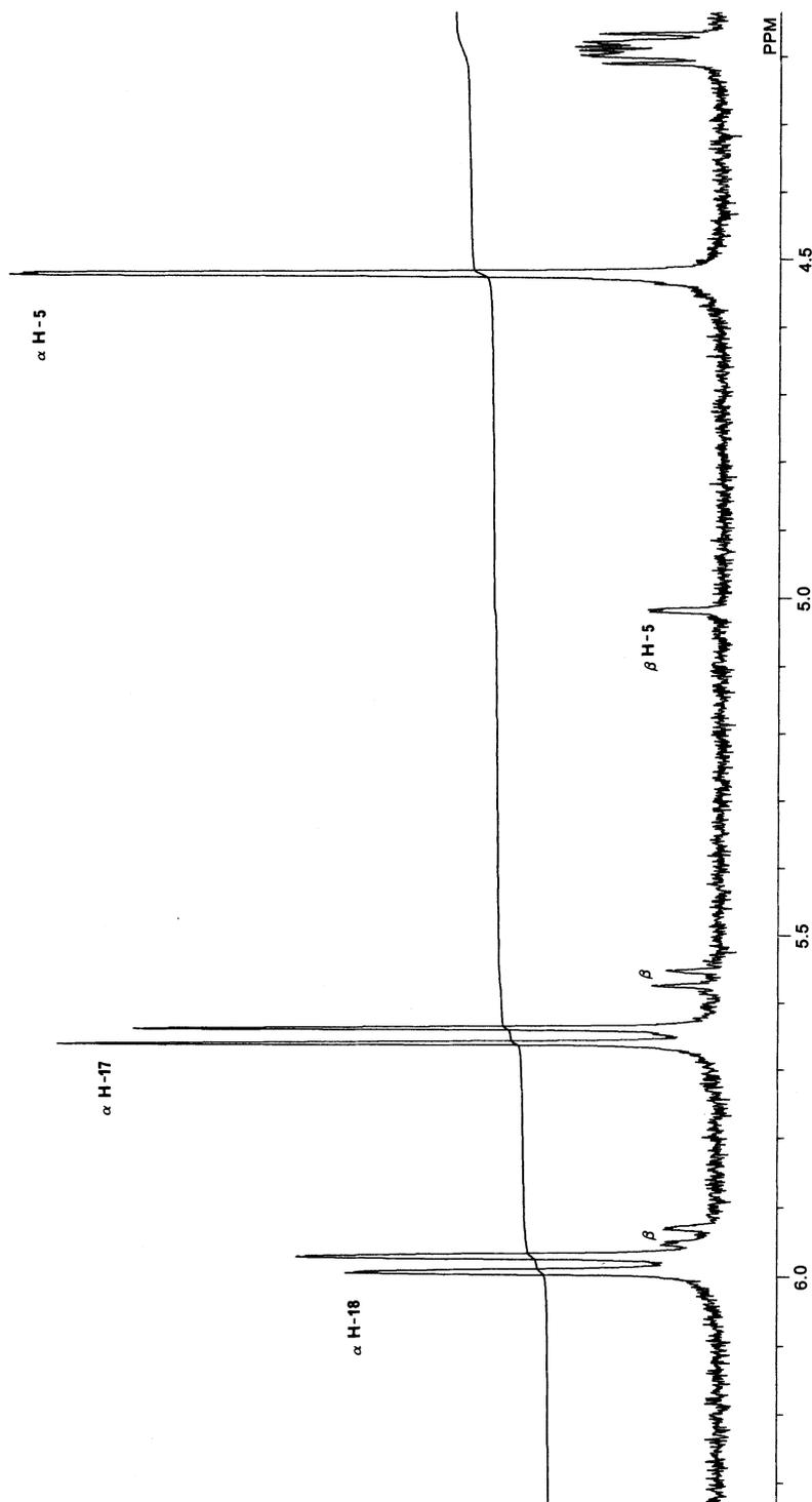
**FIGURE 13.1.** Part of the 400-MHz <sup>1</sup>H-NMR spectrum of the thebaine-acrylonitrile adduct (**29**, R = CN, 3-OMe) mixture in CDCl<sub>3</sub>. Resonances due to the major (α) and minor (β) components are annotated: H-18 and H-17 are the vinylic protons, and H-5 that attached to C-5 (see **29**).
