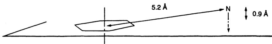
FIGURE 12.1. Pharmacophore of the 5-HT<sub>1A</sub> agonist recognition site (after Hibert *et al.*).<sup>(74)</sup>
