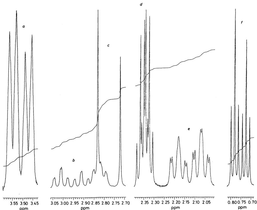
**FIGURE 13.2.** Parts of the 400-MHz  $^1\text{H-NMR}$  spectrum of ketobemidone HCl (**74b**) in  $\text{D}_2\text{O}$  showing epimeric signals due to (a) eq 2,6-H; (b) ax 2,6-H; (c) N-Me; (d)  $\text{OCH}_2\text{Me}$ ; (e) ax 3,5-H; (f)  $\text{OCH}_2\text{Me}$  (after Casy *et al.*).<sup>(177)</sup> Differing degrees of expansion have been used.
