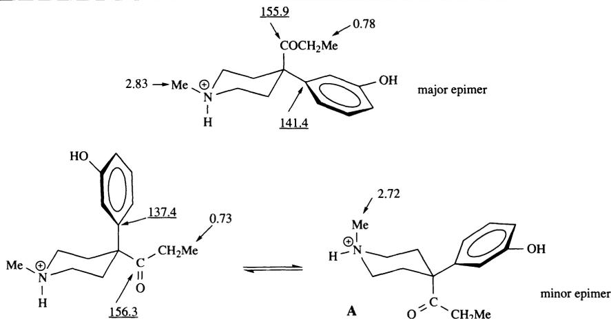
**Scheme 13.5.** N-Protonated epimers of ketobemidone:  $^1\text{H}$ - and  $^{13}\text{C}$ -NMR assignment ( $^{13}\text{C}$  values underlined).
