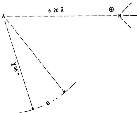
**FIGURE 11.6** Suggested pharmacophore geometry for optimum antihistaminic activity. A and B indicate the centers of gravity of Ring A and Ring B, respectively. The spreading of the N–A–B angle is that actually found (after Borea *et al.*).<sup>(100)</sup>
