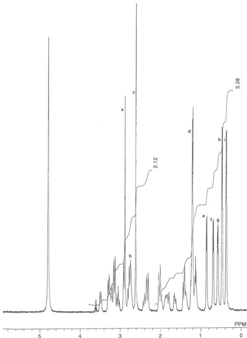
**FIGURE 13.3.** Part of the 400-MHz  $^1\text{H-NMR}$  spectrum of *trans*-1,3-dimethyl-4-(3-hydroxyphenyl)-4-isobutylpiperidine ( $\alpha$ -**83b**) hydrochloride in  $\text{D}_2\text{O}$ . Annotated epimeric resonances: (a, c) N–Me; (b) multiplet including major 3-H; (d) major 3-Me; (e, f) minor  $\text{CH}_2\text{CHMe}_2$ ; (g) minor 3-Me; (h, i) major  $\text{CH}_2\text{CHMe}_2$  (after Casy *et al.*).<sup>(192)</sup>
