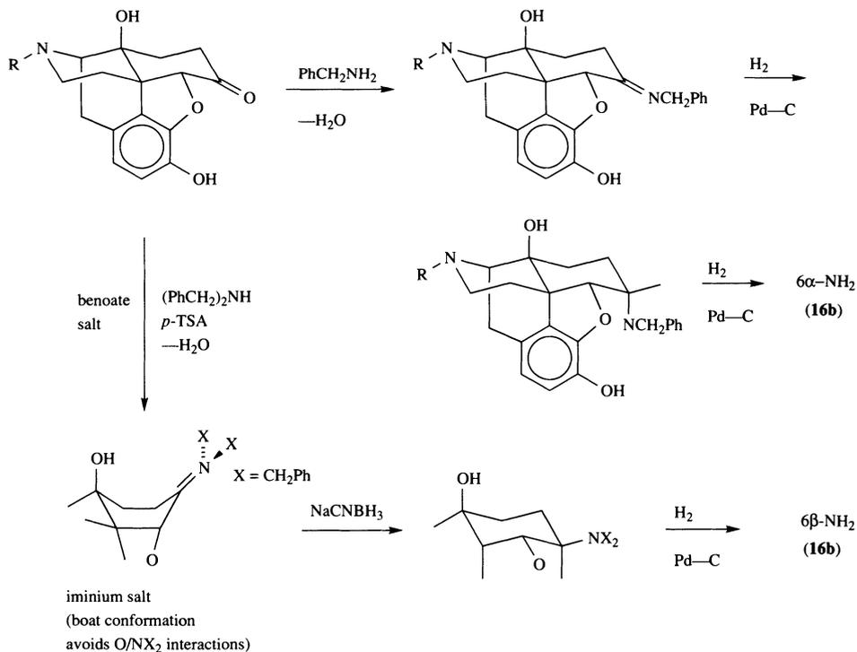
**Scheme 13.2.** Stereospecific synthesis of 6 $\alpha$ - and 6 $\beta$ -naltrexamine ( $\text{R} = \text{CH}_2\text{C}-\text{C}_3\text{H}_5$  in formulas shown).<sup>(5)</sup>
