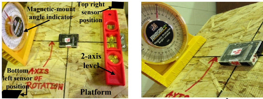
(a) Rotating platform setup (b) Sensor testing at 45° rotation
