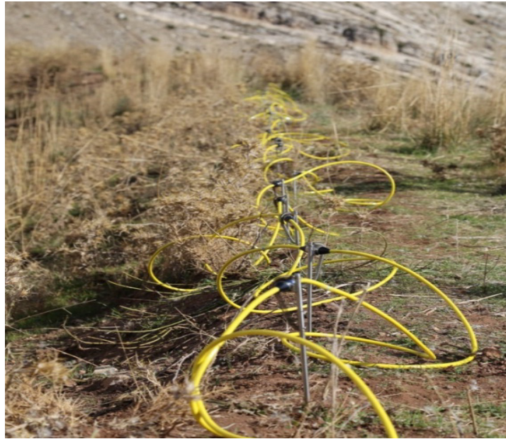
FIG. 2 Field electrical resistivity setup
