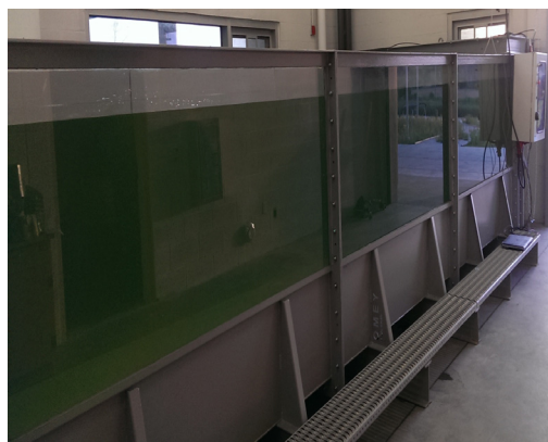
FIG 2. Omey Labs wave tank used for all wave tank testing Acoustic Wave Gauges
