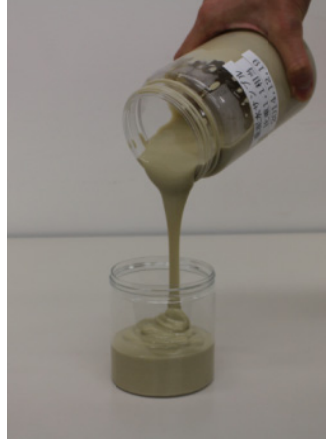
FIG.3. Picture of heavy bentonite based slurry
