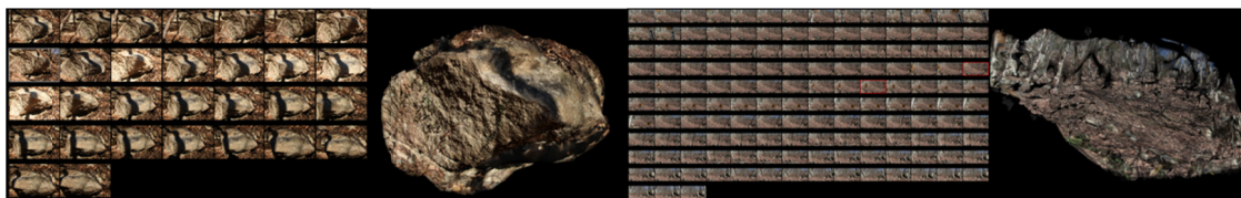
FIG. 8. Multiple-view Images and the reconstructed 3D models at Syosenkyo ((a): rock, (b): slope).
