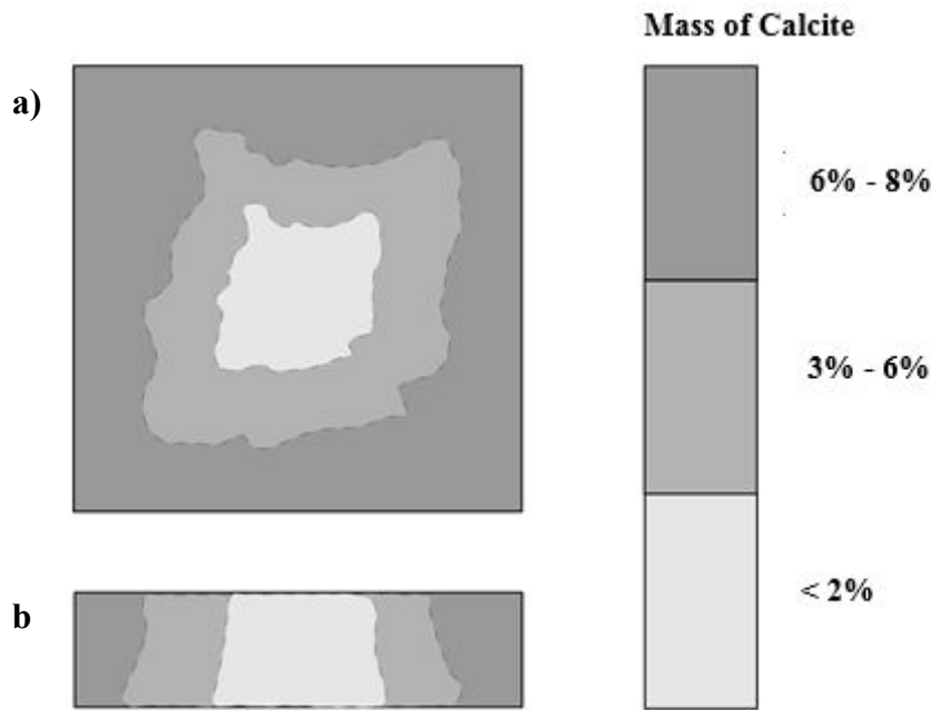
FIG 7. Cementation Distribution: a) Plan view of soil surface, b) Profile view along centerline.
