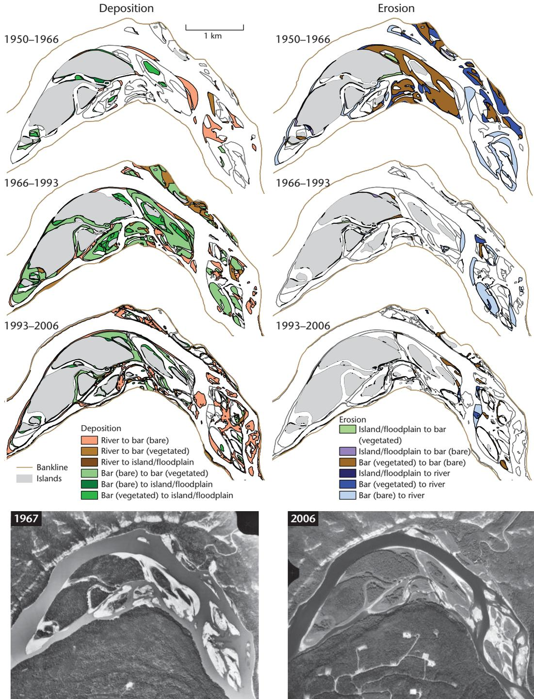
**Figure 7.5** Morphological changes between 1953 and 2006 at Many Islands (Reach AB1.4, “Many Islands”). Map panels are arranged as in Figure 7.4. Vertical air photos illustrate the site in 1964 (AS928-21; September 15,  $Q \sim 1480 \text{ m}^3\text{s}^{-1}$ : left) and 2005 (AS53788-143; August 25,  $Q \sim 710 \text{ m}^3\text{s}^{-1}$ : right) at approximately the same scale (Alberta Crown copyright).
