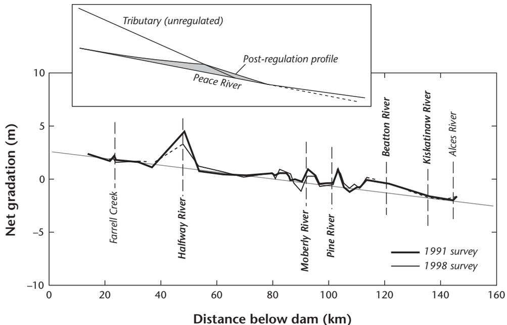
**Figure 3.12** Schematic diagram showing the development of a stepped long profile in the British Columbia reach of Peace River. Note the backwaters and steepened reaches at aggradation zones. Vertical scale greatly exaggerated. Inset: sketch of the characteristic situation at a prograding tributary junction (see also Ferguson and Hoey, 2008, Figure 10.6b, which presents a simulation of the same effect).
