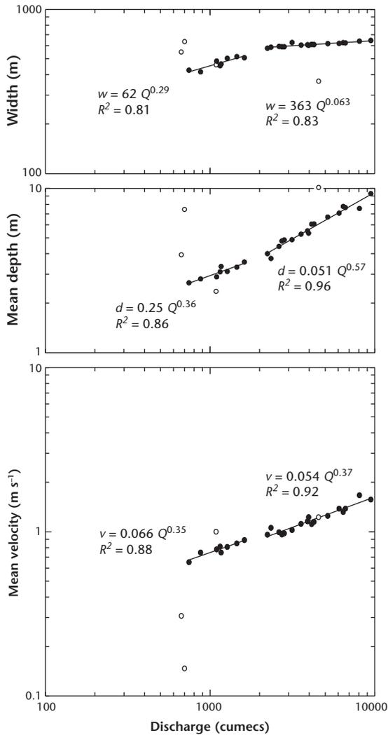
**Figure 5.12** Open-water hydraulic geometry for WSC Stn. 07HD001, Peace River at Carcajou for the pre-regulation period 1961 to 1967, segmented into “high-flow” and “low-flow” subsets. Aberrant data (open symbols) are plotted but not included in the calculation of the best-fit functions.
