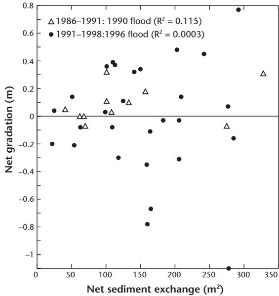
**Figure 10.6** Gradation in the British Columbia reach in 1990 and 1996. Net gradation at monumented cross-sections is plotted against net sediment exchange. For 1990, only cross-sections below the Pine confluence are plotted.
