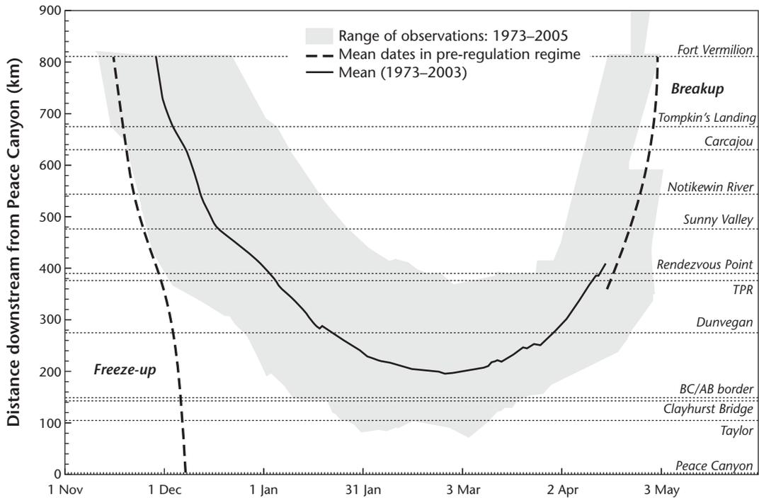
**Figure 6.2** Location and date of the ice front on Peace River (the mean and range of dates for 1973 to 2005 are from Jasek *et al.*, 2007), from which the diagram is adapted).
