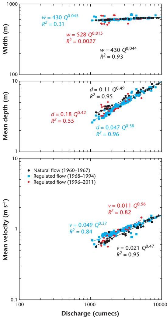
**Figure 5.16** Open-water hydraulic geometry for Peace River at Peace Point. Significant change was induced by the moderate but long-sustained flood of 1996.
