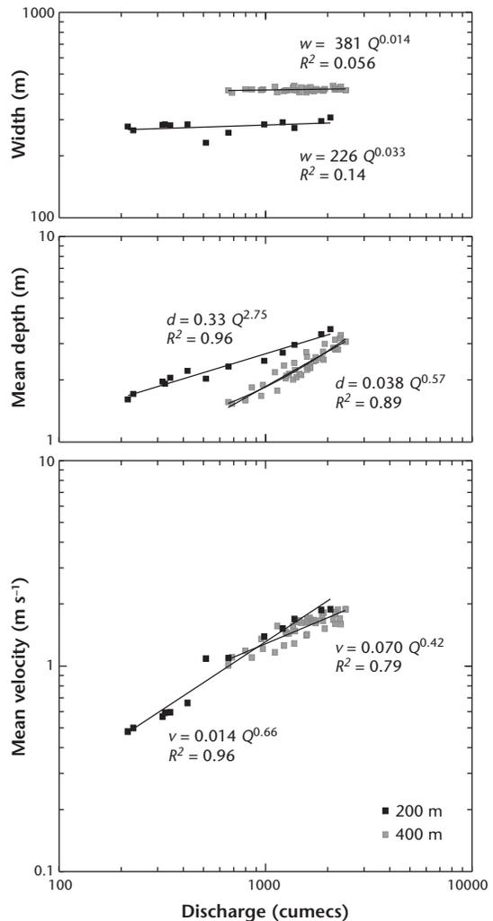
**Figure 5.7** WSC Stn. 07FD002, Peace River at Taylor: hydraulic geometries for open water, period 1968 to 1995. Distinct geometries for a 250 m wide river and for a 400 m wide river are displayed. Two outlying data from the 1972 spillway flood are deleted.
