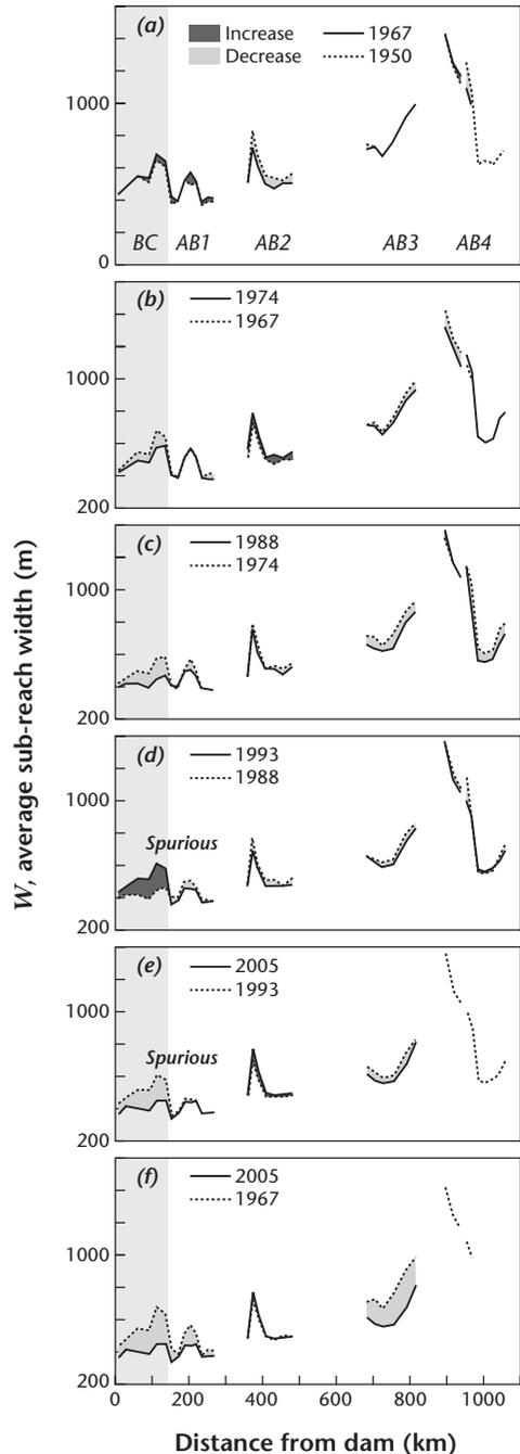
**Figure 7.17** Spatial trends in channel width along Peace River displayed as cumulative change at the end of each survey period. Panel f indicates net change since regulation. The indicated changes in panels d and e for the BC reach should be disregarded because of high flows at the time of the 1993 photography. Reach AB4 data are incomplete due to limited air photo coverage.
