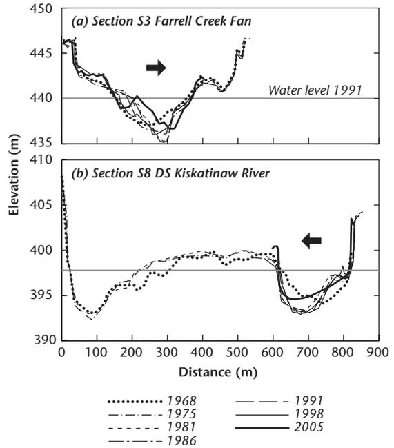
**Figure 3.7** Cross-section histories at sections on prograding fans: (a) Farrell Creek (section S3); (b) Kiskatinaw River (section S8). Arrows indicate the direction of fan progradation.
