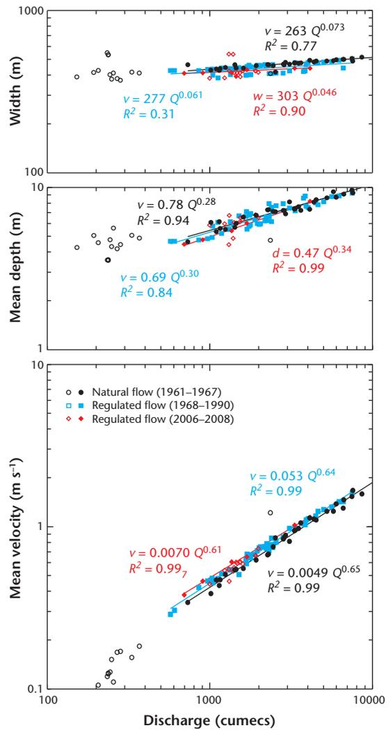
**Figure 5.13** WSC Stn. 07HF001, Peace River at Fort Vermilion, data for 1961 to 2011. All data are shown: displayed equations are based on a subset excluding ice period measurements (open symbols) and one aberrant datum. Displayed equations describe open-water hydraulic geometry for Peace River at Fort Vermilion for three periods.
