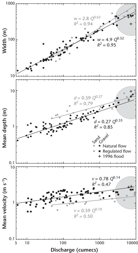
**Figure 5.18** The hydraulic geometry of Albertan rivers (After Bray (1973) and Neill (1973)) showing Peace River data, which are inside the shaded circle. See text for details of the derivation of the Peace River data.
