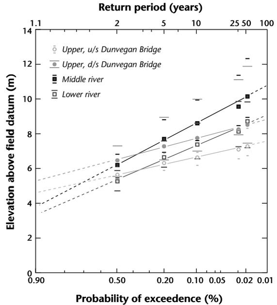
**Figure 6.8** Elevation-frequency plots for ice-jam stages in major reaches of Peace River. The upper river is represented by two plots because of the noted relatively low elevations and transient freezing above Dunvegan. Error bars represent 5% and 95% confidence limits on the estimated elevations.
