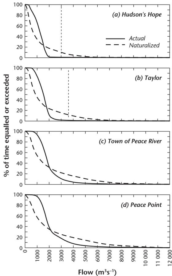
**Figure 2.15** Flow duration curves for the period 1972 to 1999 compared with “naturalized flows”—the flows it is estimated would have occurred in the period if the dams had not been present. Vertical line indicates a nominal competence criterion for gravel entrainment from the bed in the upper river. See text for further details (Naturalized flows courtesy of British Columbia Hydro and Power Authority; analysis by C. P. Ayles).
