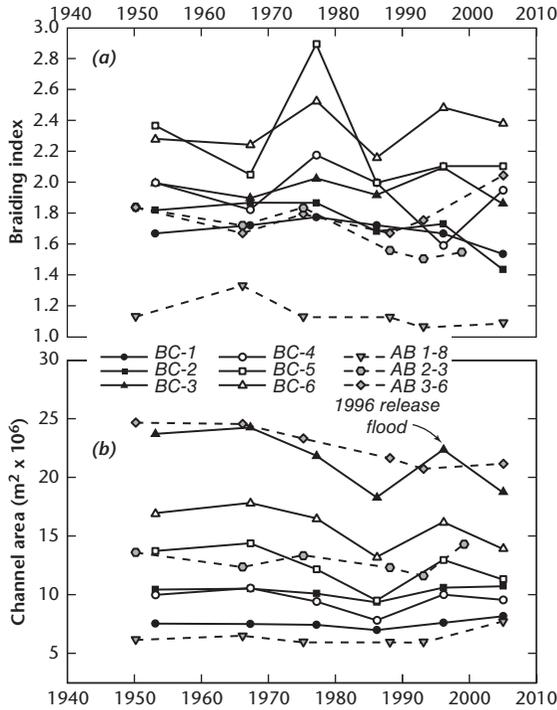
**Figure 3.6** (a) First braiding index; (b) Channel area, by principal sub-reach. British Columbia data are recorded by sub-reach. Alberta data are given only for the gauge sub-reaches (AB1-8, Dunvegan; AB2-3, TPR; AB3-6, Fort Vermilion; no morphological data are available for Peace Point).
