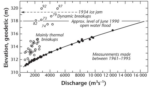
**Figure 2.14** Peak water level versus discharge at the Town of Peace River (WSC Stn. 07HA001). Closed symbols and curve indicate the open water discharge measurements and stage-discharge relation. Open symbols indicate extreme ice-induced high water; and post-regulation years are identified. No flow datum is available for the 1934 ice jam (Analysis by L. Uunila).
