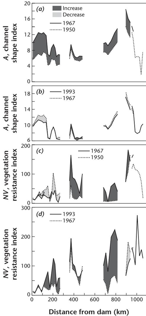
**Figure 7.21** Spatial trends in flow resistance factors along Peace River: (a) and (b) channel shape index; (c) and (d) vegetation index.
