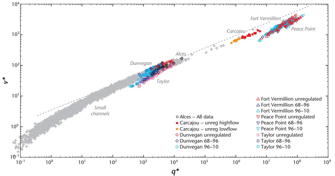
**Figure 5.21** Dimensionless hydraulic geometry to demonstrate the coherence of flow resistance along Peace River. Range of data plotted by Rickenmann and Recking (2011) is shown as gray spots; Peace River stations are individually distinguished for individual periods before and after regulation. The dashed line is Ferguson’s deepwater limit equation, based on the Manning–Strickler relation.
