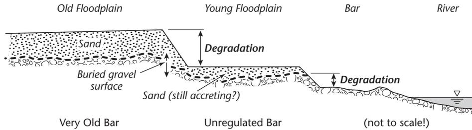
**Figure 4.3** Schematic diagram of the methods for estimating tributary degradation by surveying floodplain and bartop levels, showing old (i.e., pre-regulation) floodplain; young (post-regulation) floodplain; old and active bartops.
