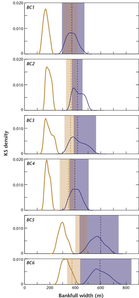
**Figure 11.3** Single-thread regime predictions for six sub-reaches in the BC reach of Peace River. The distribution of post-regulation single-thread channel widths predicted by the UBCRM is displaced to the left of the measured pre-regulation distribution. The distributions are shown as smoothed density plots while the medians and interquartile ranges are shown as vertical lines (median value) and shaded regions (interquartile range); the post-regulation predicted range is cross-hatched.
