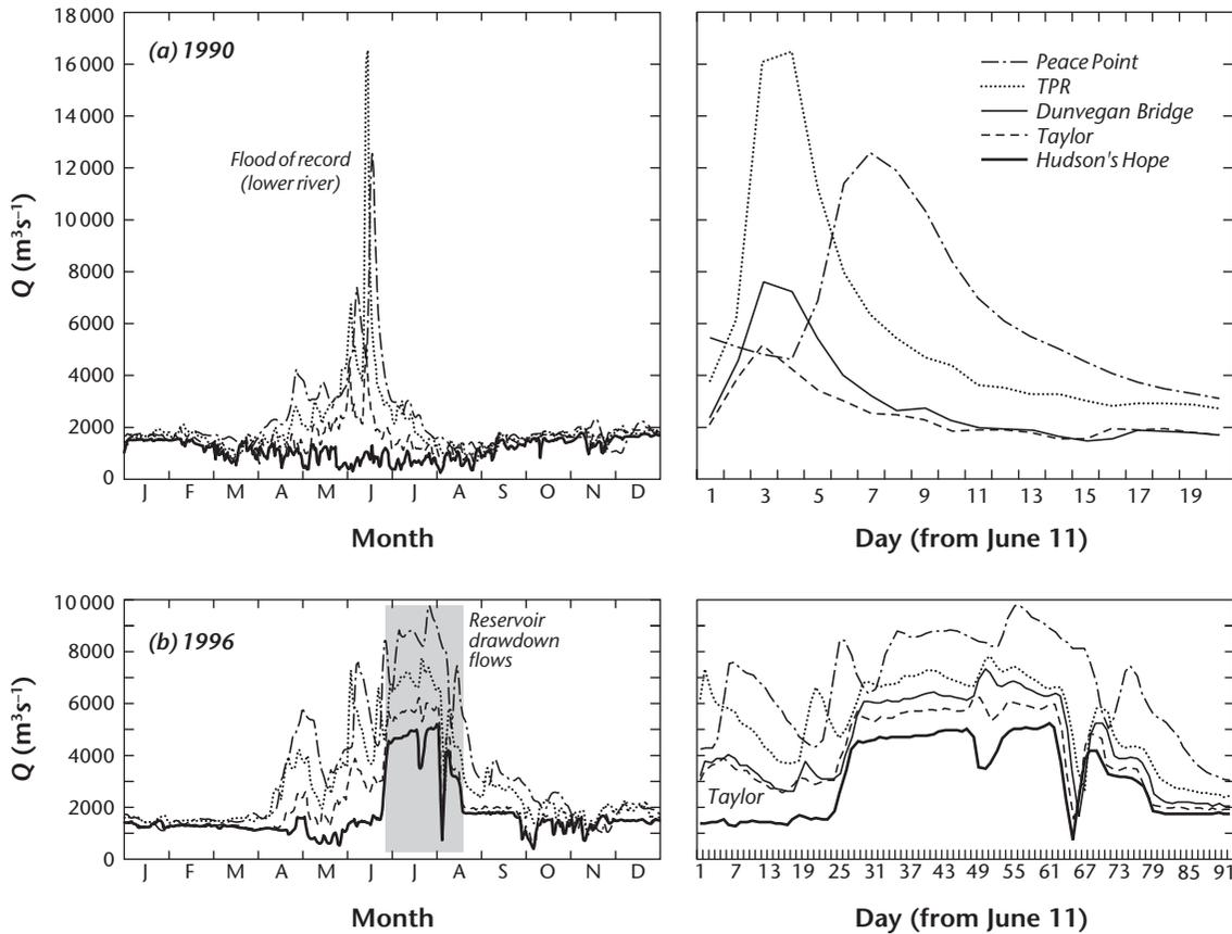
Figure 10.3 Annual and flood event hydrographs for principal stations for (a) 1990 and (b) 1996. See Figure 10.2 for gauge locations.
