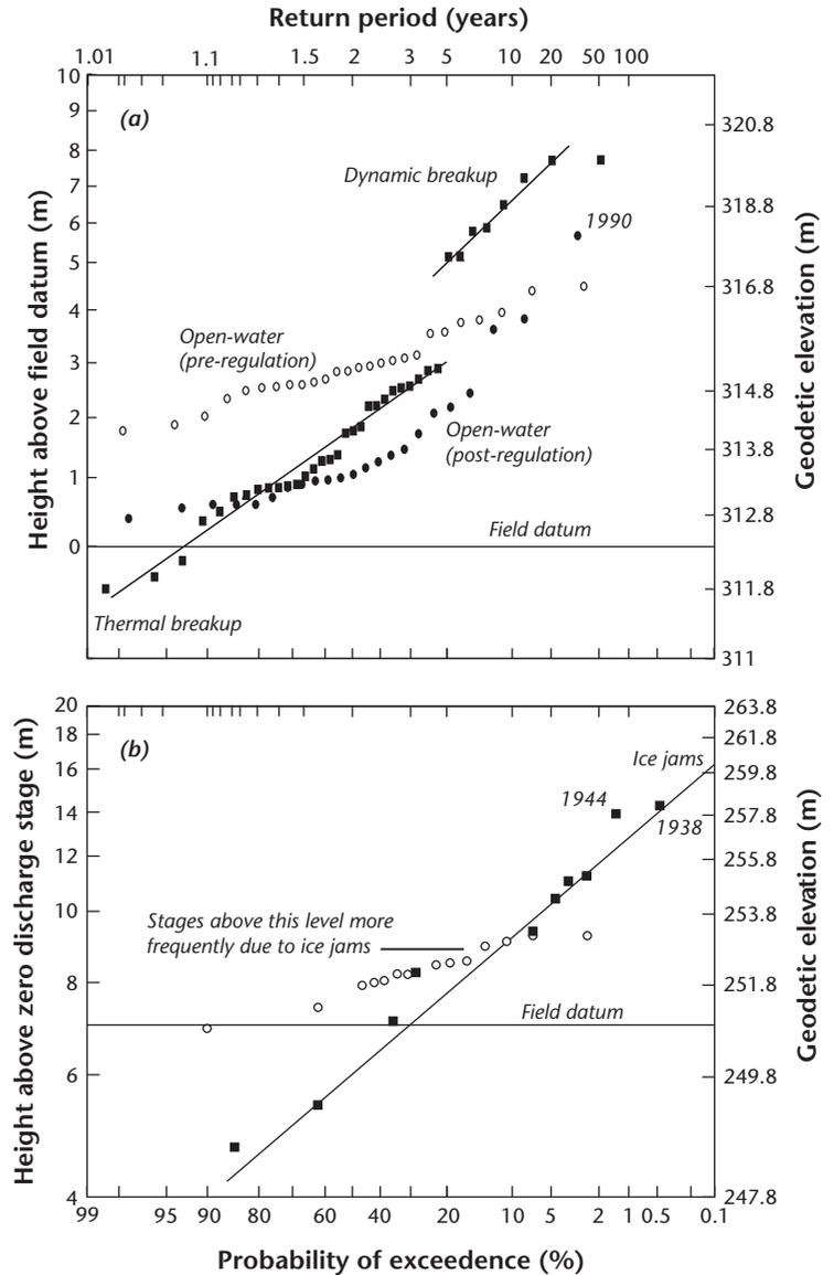
**Figure 6.9** Historical ice-jam stages in comparison with open-water stages at (a) Town of Peace River and (b) Fort Vermilion. The Fort Vermilion record is for the pre-regulation period. The gauging record extends from 1917 to 1922 and from 1961 to 1968. The ice-jam record extends back to 1920, but includes records from only some years. The ice stage records at TPR include all available data, before and after regulation.
