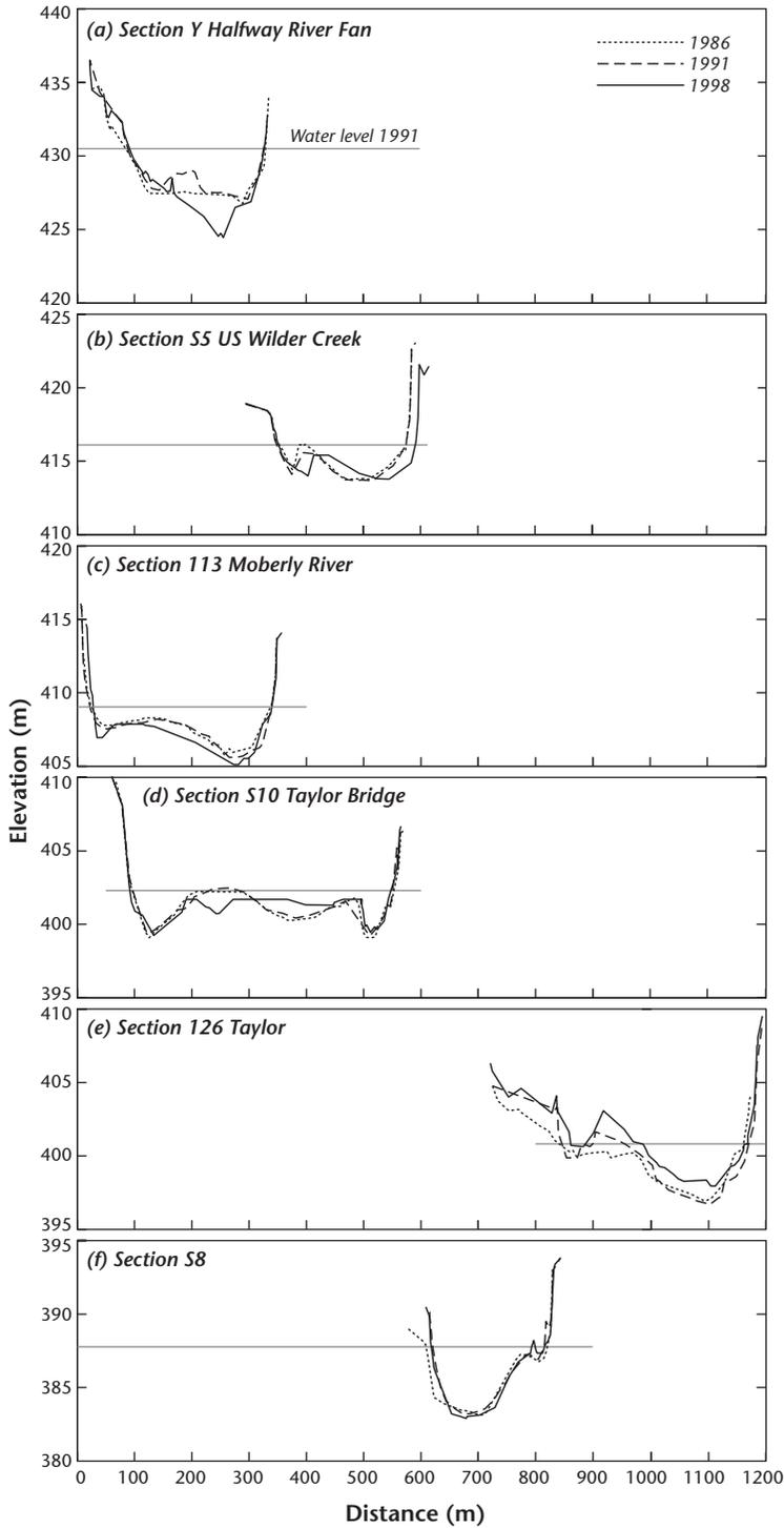
**Figure 10.5** Selected surveyed cross-sections in the British Columbia reach of Peace River to illustrate the contrasting effects of the 1990 and 1996 floods. Panels (a) to (c) are from sections above the confluence of Pine River, panel (d) shows the section immediately below the confluence, and panels (e) and (f) are from farther downstream.
