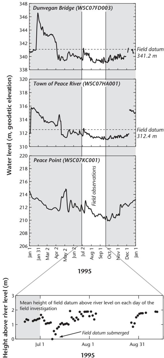
**Figure 6.6** Water level variations at Dunvegan and TPR gauges during the field survey and the elevation of field datum above river level. Data for Peace Point are also shown as the Carcajou and Fort Vermilion gauges were inactive in 1995.
