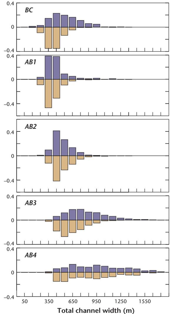
**Figure 11.2** Distribution of observed total channel widths along five reaches of Peace River. In each panel, the pre-regulation distribution is shown in the upper histogram, and the post-regulation distribution is shown in the lower one.
