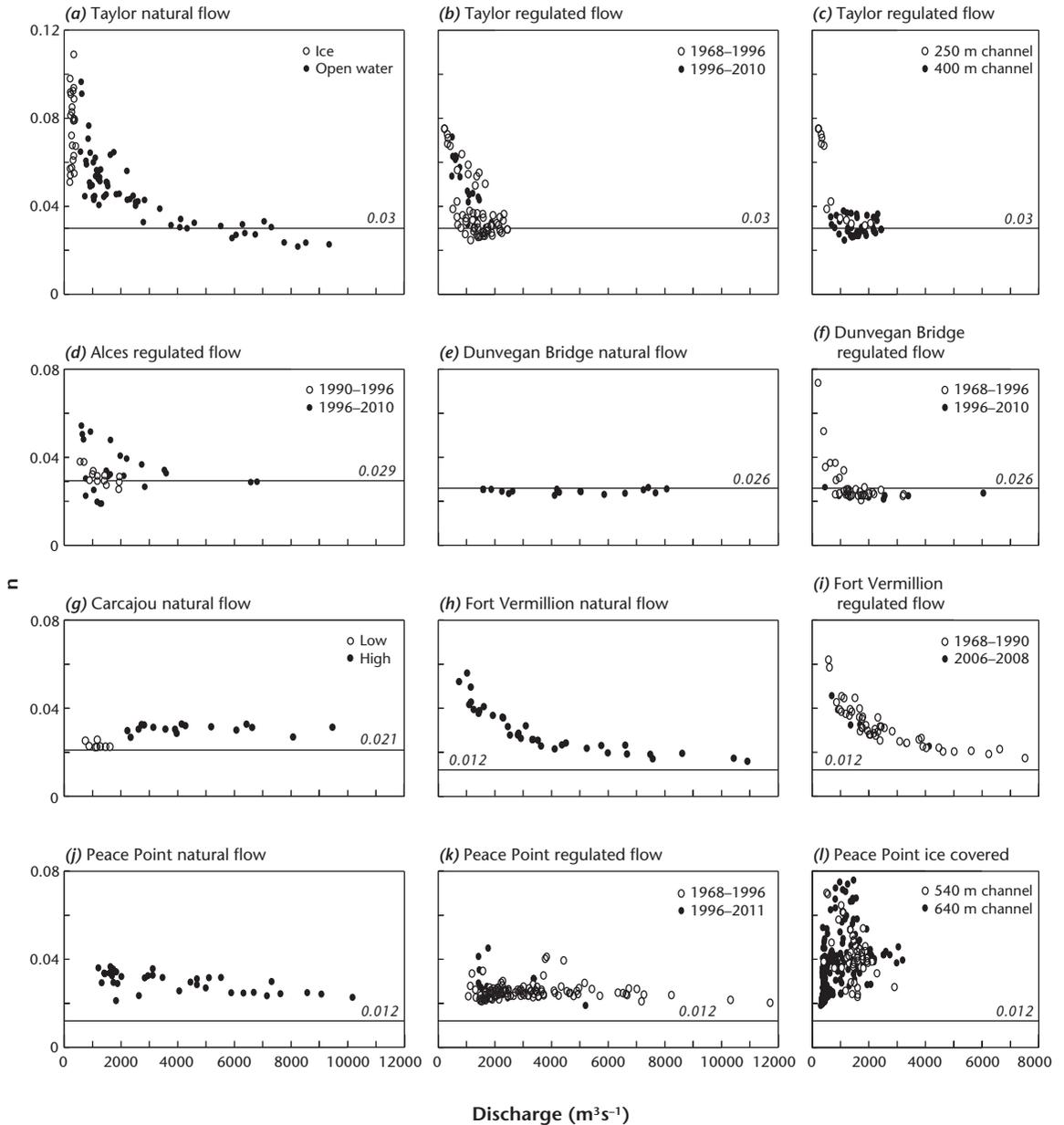
**Figure 5.20** Pattern of variation of Manning’s  $n$  at gauging stations on Peace River. In each panel, the annotated horizontal line indicates the lower limit dictated by grain size using Strickler’s relation.
