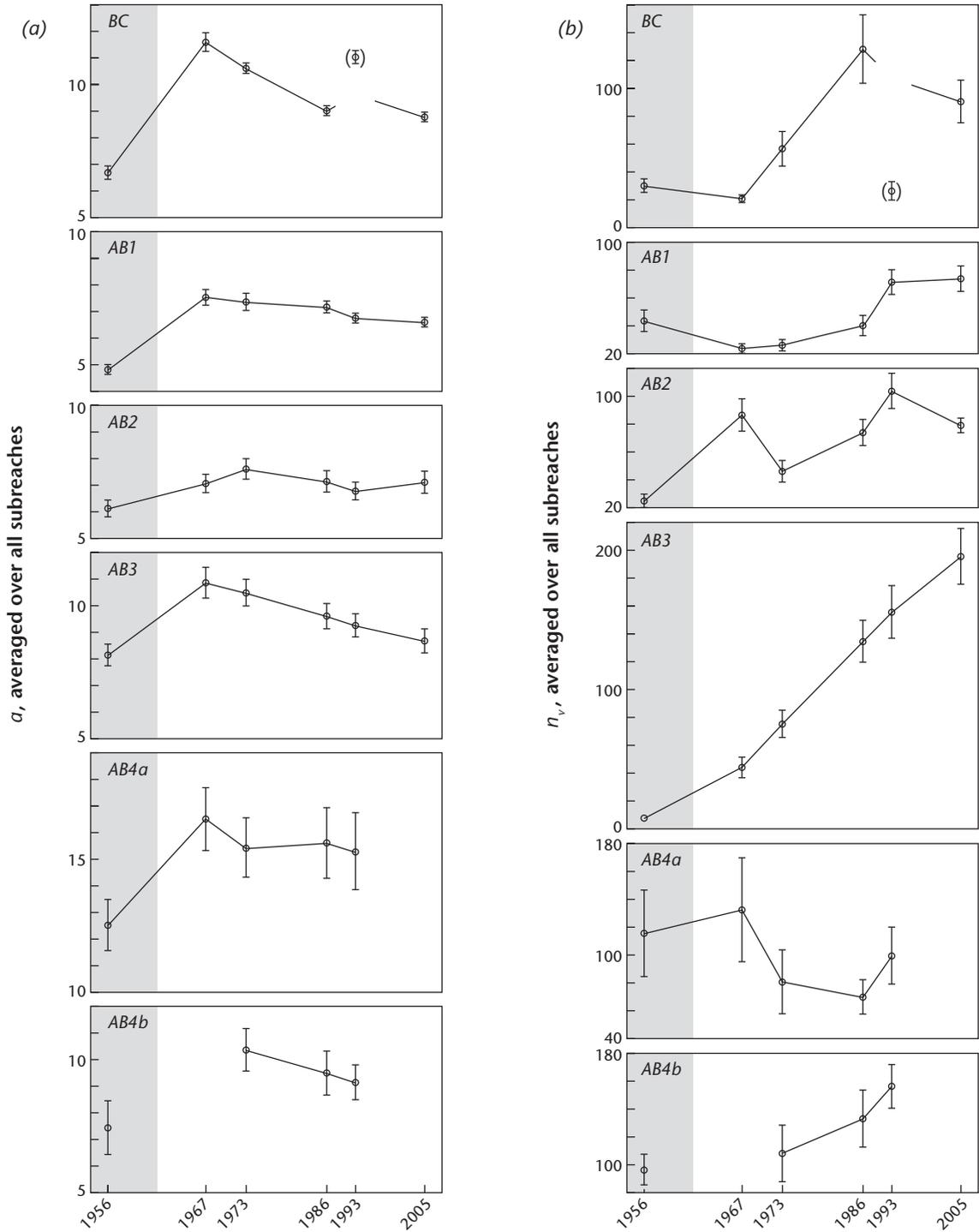
**Figure 7.20** Reach-level temporal trends in the controlling factor indices along Peace River: (a) channel shape index; (b) vegetation index. The error bars represent 2s ranges of variance based on sub-reach data. The grey background indicates the period before regulation. The connecting lines are to aid comprehension of the pattern of change and are not meant to imply linear trajectories of change between data.
