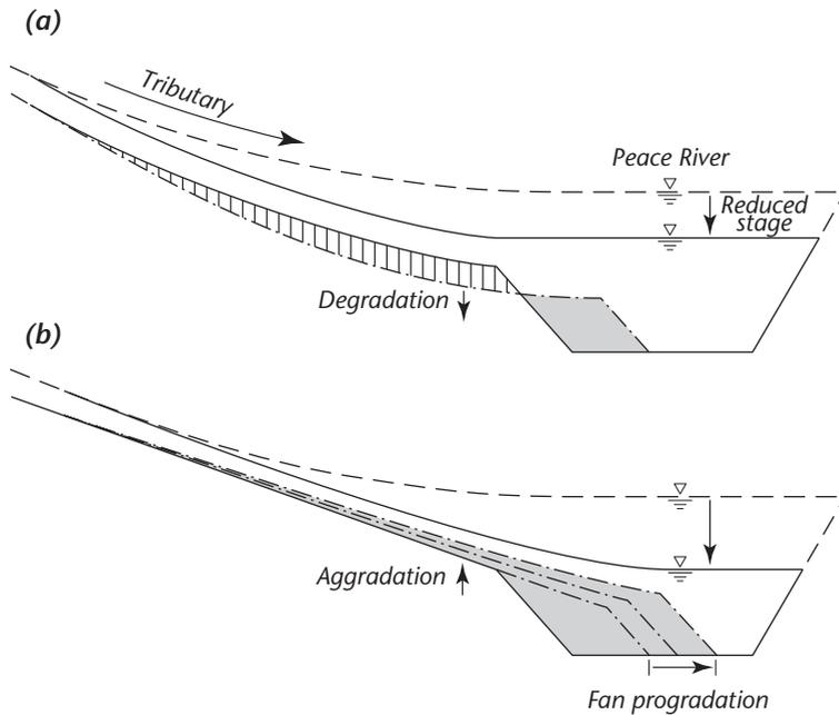
**Figure 4.2** Lower tributary gradation scenarios following mainstem regulation: (a) degradation due to reduced water levels in the mainstem; (b) aggradation due to tributary fan progradation. Peace River is viewed in cross-section, the tributary in longitudinal section.
