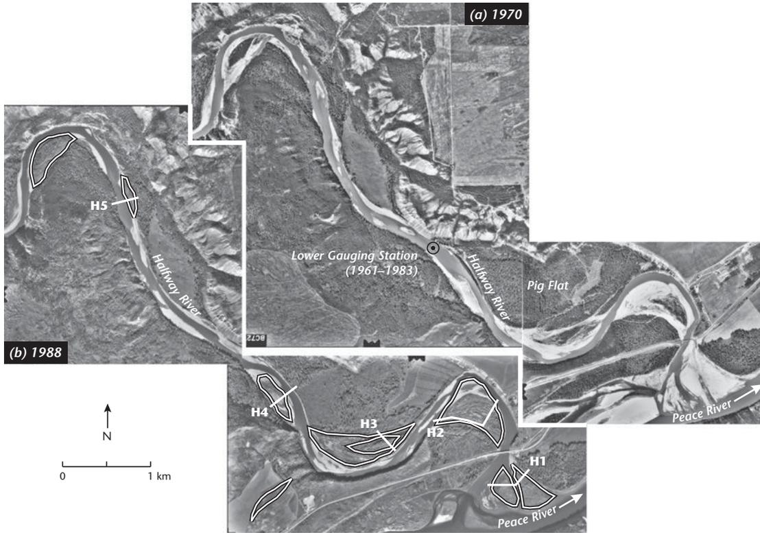
**Figure 4.6** Historical aerial photographs of Halfway River (a) shortly post-dam (photos BC7279-070 and 118), and (b) in 1988 (BC88088-171 and 180). Young floodplains developed between the two dates are outlined in (b) and surveyed transects are labeled (Ayles, 2001, Figure 3.10, p. 88).
