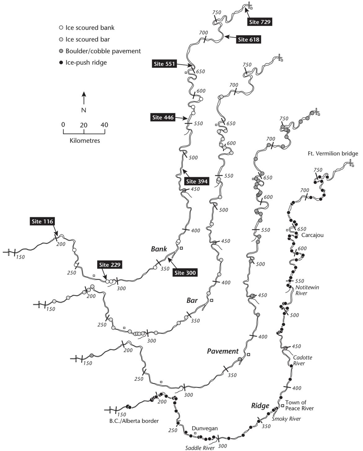
**Figure 6.10** Distribution of ice-associated sedimentary features along Peace River. Features mapped have a characteristic dimension of one meter or greater. Also shown, the location of bank profiles illustrated in Figure 6.14 and additional sites with data in Figure 6.12.
