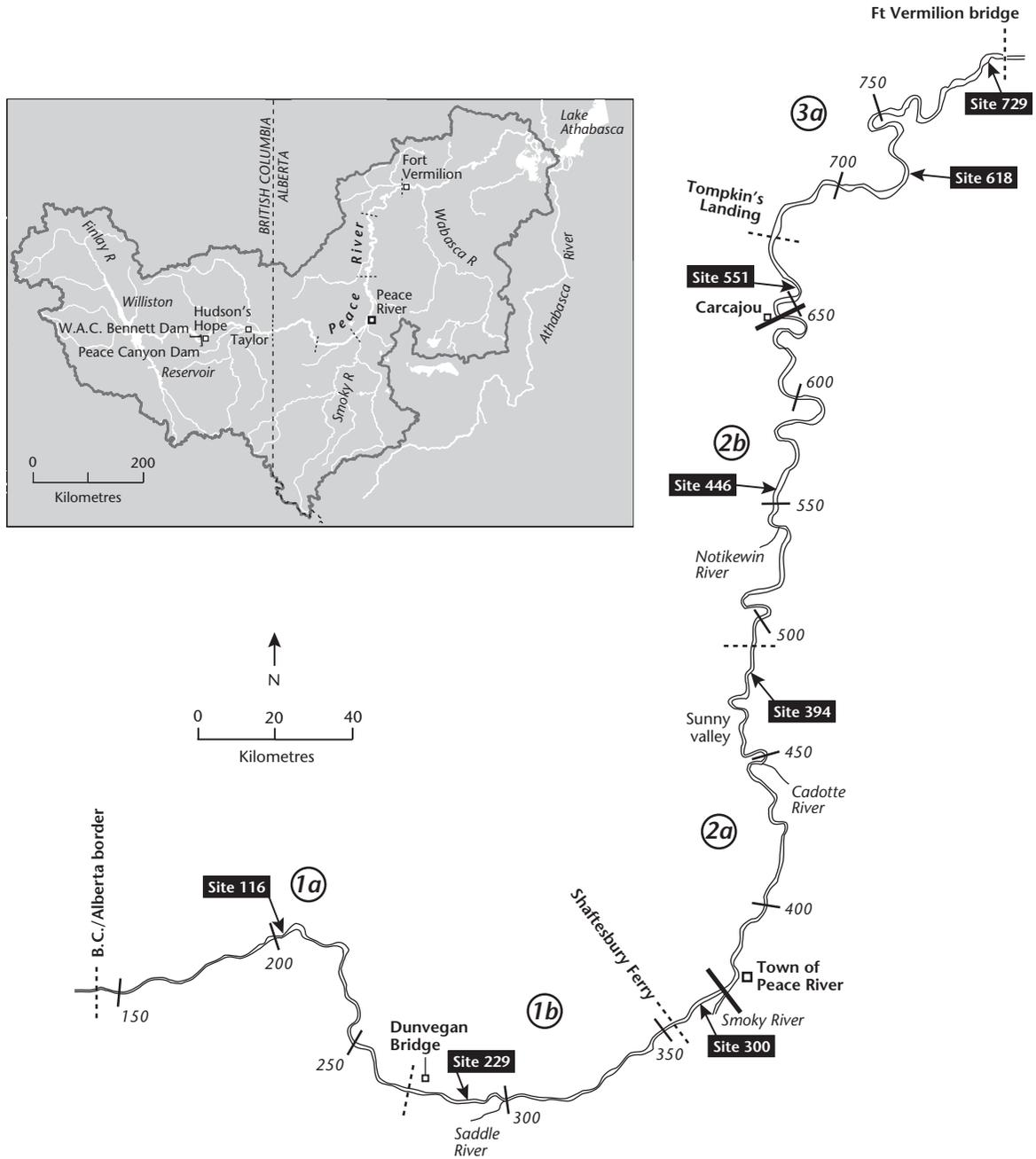
**Figure 6.1** Map of Peace River in Alberta, showing the reaches established for analysis of the ice regime and the location of bank profiles illustrated in Figure 6.14 and data plotted in Figure 6.17. Numbers along the river are distance in kilometers below the Peace Canyon Dam. Bold lines mark the limits of the cobble-gravel and sandy gravel reaches. Inset: Peace River basin.
