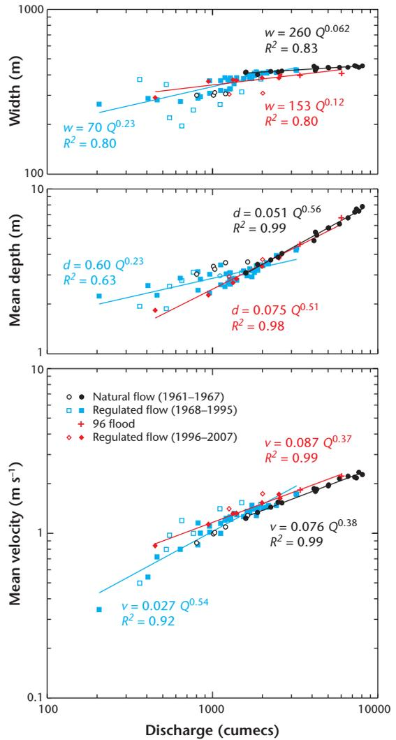
Figure 5.10 WSC Stn. 07FD003, Peace River at Dunvegan Bridge, for the period 1961 to 2007: mass plot of data and hydraulic geometry for three periods: aberrant data (open symbols) are plotted but not included in the calculation of the best-fit functions. Measurements taken during the 1996 flood are annotated.
