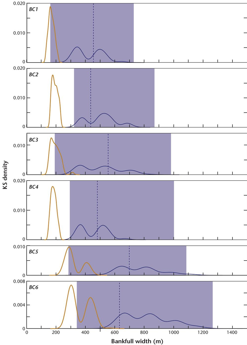
**Figure 11.5** Regime-based predictions of channel pattern and total channel width for six sub-reaches in the BC reach of Peace River. The distribution of pre-regulation measured and post-regulation predicted widths (dashed line) are shown as smoothed density plots. The median and interquartile range of the total pre-regulation channel width distribution are shown using a line and shaded area, respectively.
