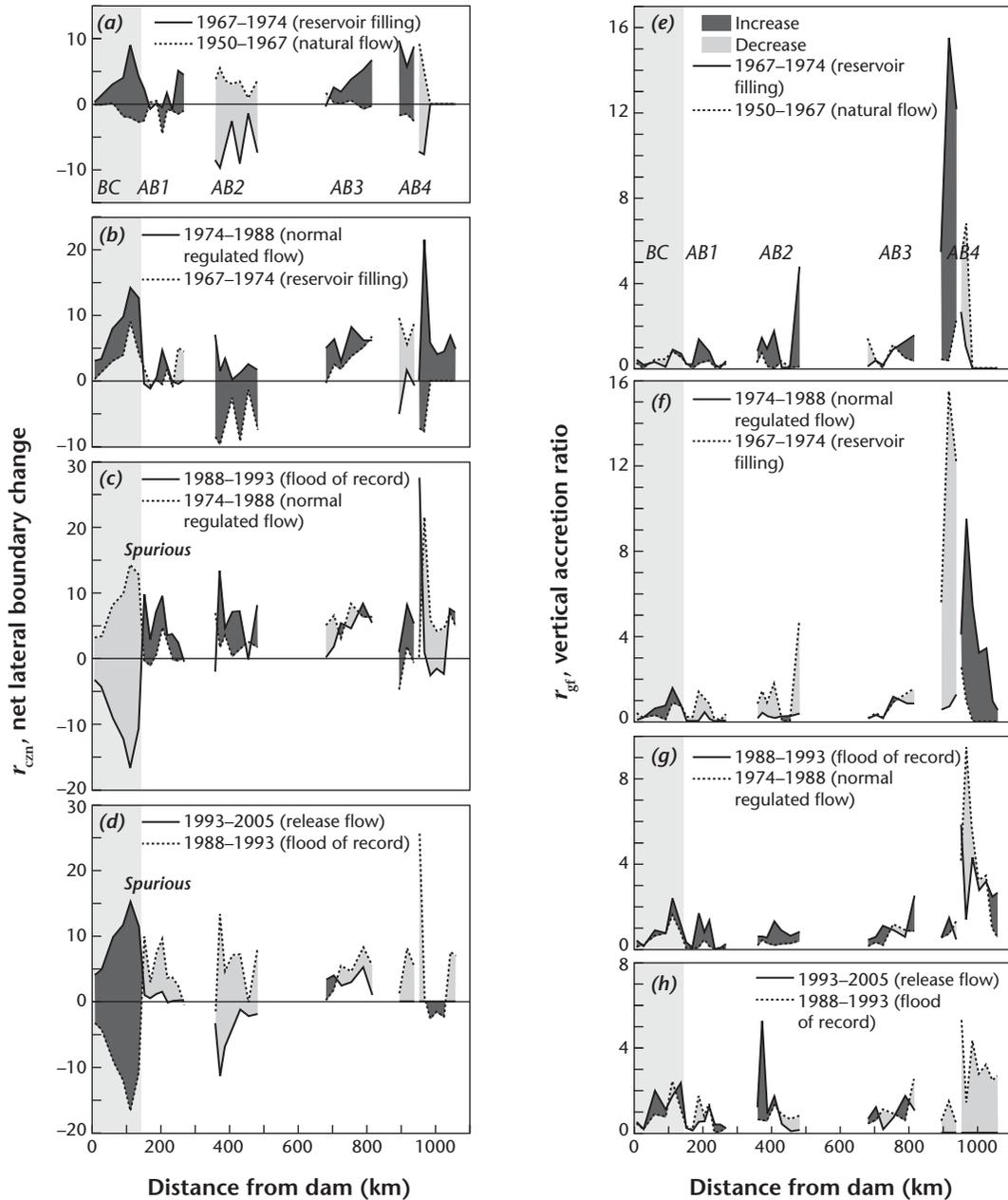
**Figure 7.19** Period-to-period comparison of indices of channel change:  $r_{czn}$ , the index of lateral channel erosion/accretion;  $r_{gf}$ , the index of vertical accretion. Positive values indicate net accretion (channel narrowing) and net floodplain production. These charts show the change in the indices from one inter-survey period to the next. Therefore the graphs indicate changes within periods, not conditions at absolute dates.
