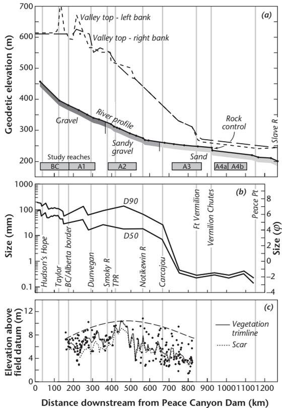
**Figure 7.2** Long profile of Peace River, showing (a) the river entrenchment, (b) surface bed material grain size, and (c) the upper envelopes of ice damage (upper limit of damaged trees) and 20-km running averages of tree damage and of scar tissue (Chapter 6). The location of the study reaches is also shown.
