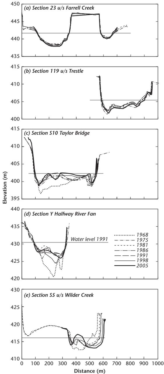
**Figure 3.2** Cross-section histories for 38 years of regulated flows, illustrating typical patterns of channel gradation: (a) Section 23: stable; (b) 119: aggrading; (c) S10: aggrading; (d) Y: fan progradation; (e) S5: scour/fill.
