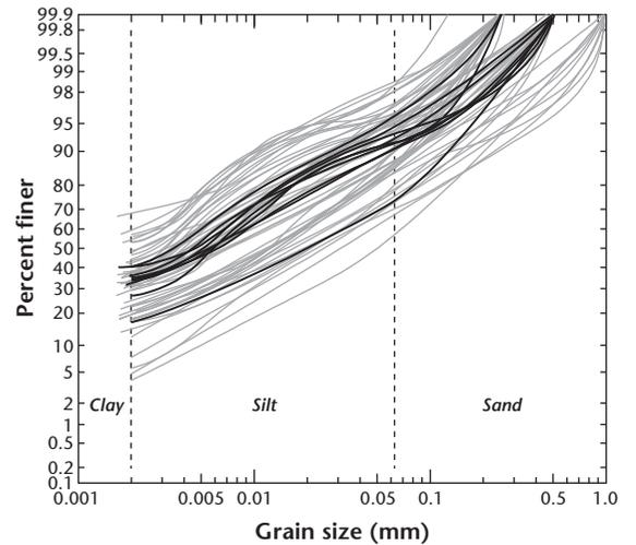
**Figure 2.17** Mass plot of grain size distributions of suspended sediments from the British Columbia reach of Peace River and its principal tributaries. Note the strongly nonlinear ordinate axis. There are between 2 and 11 curves for each station. Most analyses derive from composites of several individual water samples. The emphasized curves are from Peace River below Alces River; that is, at the British Columbia–Alberta border (Data from BC Hydro (1975)).
