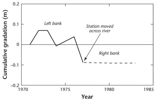
**Figure 4.7** Halfway River specific gauge analysis for the lower station (WSC Stn. 07FA001). Results are for  $Q = 578$  m<sup>3</sup>s<sup>-1</sup>.
