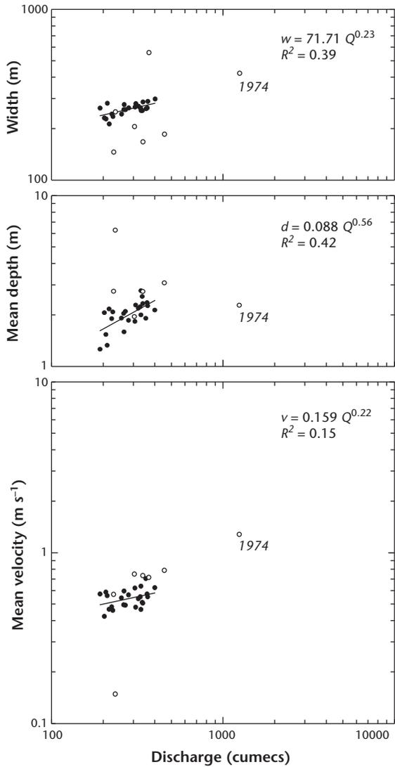
**Figure 5.4** WSC Stn. 07FD002, Peace River at Taylor: hydraulic geometry with ice on the river, period 1945 to 1969, natural regime and the first two winters of flow regulation (reservoir filling; flows extremely low). Aberrant data are plotted (open symbols) but not included in the calculation of the best-fit function.
