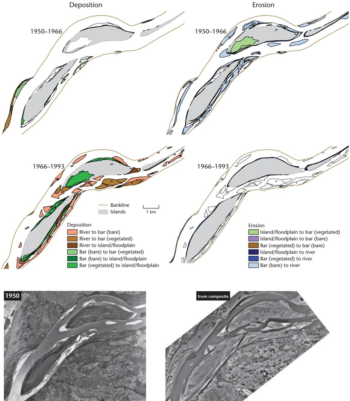
**Figure 7.8** Morphological changes between 1967 and 1993 near Fifth Meridian (Reach AB4). Map panels are arranged as in Figure 7.4. Vertical air photos illustrate the site in 1964 (AS885-131/132; June 29,  $Q \sim 7160 \text{ m}^3\text{s}^{-1}$ : left) and 1983 (AS2783-210/211; August 28,  $Q \sim 1620 \text{ m}^3\text{s}^{-1}$  (right) (Alberta Crown copyright).
