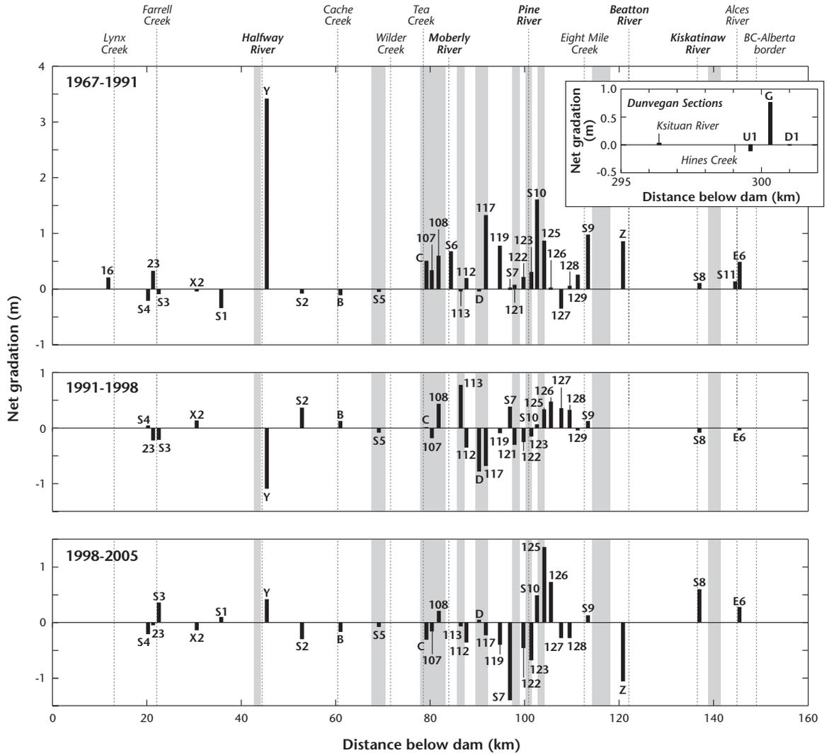
**Figure 3.3** Net gradation results to 2005. Also shown, tributaries (major sediment delivering tributaries in bold) and the location of unstable sections of valley side (grey bars), including landslides, that have recently contributed sediment to the river.
