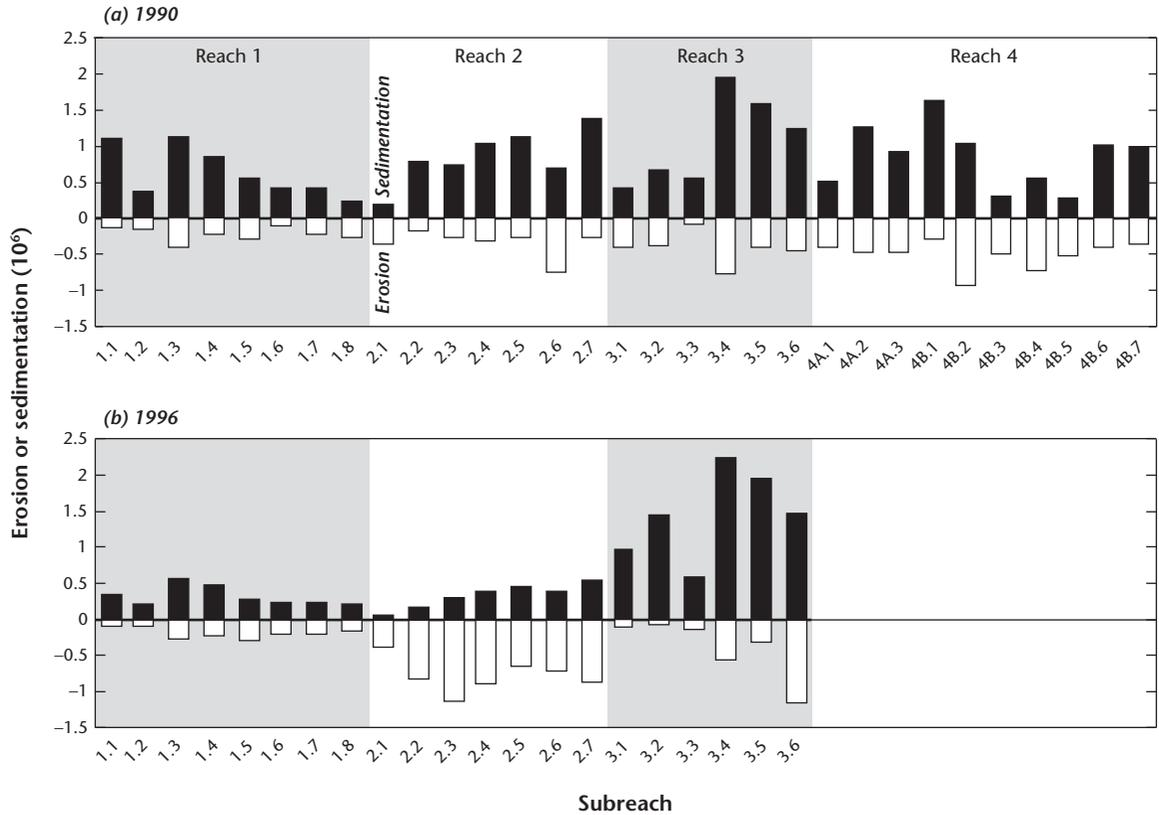
**Figure 10.10** Areal change ( $10^6 \text{ m}^3$ ) in exposed surface during the periods encompassing the 1990 and 1996 floods in the Alberta Peace River; results aggregated by study sub-reaches.
