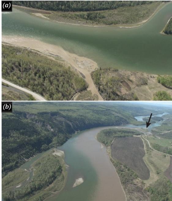
**Figure 2.18** (a) Suspended sediment entering Peace River from ungauged Farrell Creek, May 28, 2009. Farrell Creek enters Peace River 24 km below Peace Canyon Dam (Peace River flow is right to left). (b) Suspended sediment plume originating from Halfway River (arrow). View upstream, May 28, 2009; flow is  $1195 \text{ m}^3\text{s}^{-1}$  (Photo courtesy of M. J. Miles).
