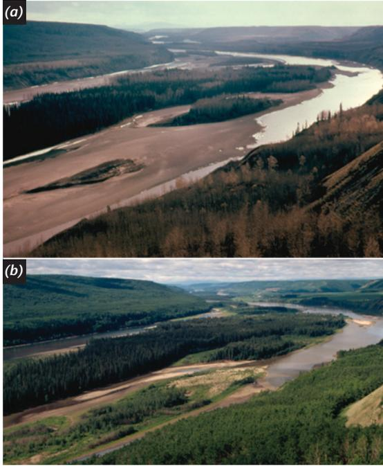
**Figure 7.13** Change in the vegetated channel zone in the British Columbia reach, views upstream near Bear Flat: (a) May 1968, extremely low flow during reservoir filling,  $Q \sim 200 \text{ m}^3\text{s}^{-1}$  (Photo courtesy of R. Kellerhals); (b) July 1998,  $Q \sim 550 \text{ m}^3\text{s}^{-1}$ . The principal channel is near the far (right) bank.
