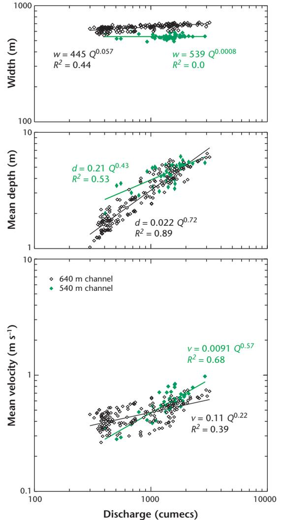
**Figure 5.15** Ice-regime hydraulic geometry for Peace River at Peace Point: two regimes are evident, one reflecting river width, the other subject to ice build-up alongshore. Ten aberrant data points have been deleted in the pre-1967 period and one in the post-1996 period. The deleted points occur in clusters of adjacent measurements, suggesting that they are the result of unusual ice configurations.
