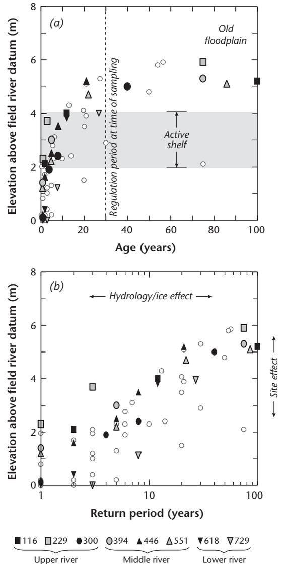
**Figure 6.17** (a) Age-elevation plots for vegetation sampled on the bank profiles of Figure 6.14 (with additional sites) and (b) derived return period plots for ice disturbance at elevations above river field datum. Locations of plotted sites are shown in Figure 6.1 and Figure 6.10. Open circles are data from additional sites along the river.
