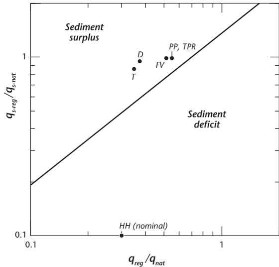
**Figure 2.24** Schmidt and Wilcock (2008) type diagram for Peace River stations downstream from the dams. The diagram has been modified to display direct observables. See text for details.
