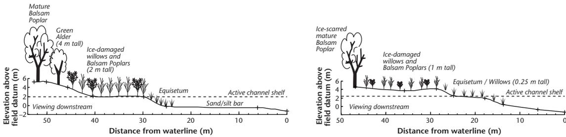
**Figure 6.14** Bank profiles in typical depositional environments along Peace River, that is, moderate- to low-exposure sites. See Figure 6.1 and Figure 6.10 for locations.
