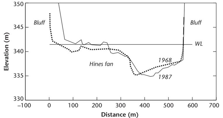
**Figure 5.11** Surveys at section U (Peace River at Dunvegan Bridge). Sediment deposition from Hines Creek has forced the channel to the right during the period of record. It is doubtful that the same survey positions were occupied on the left bank.
