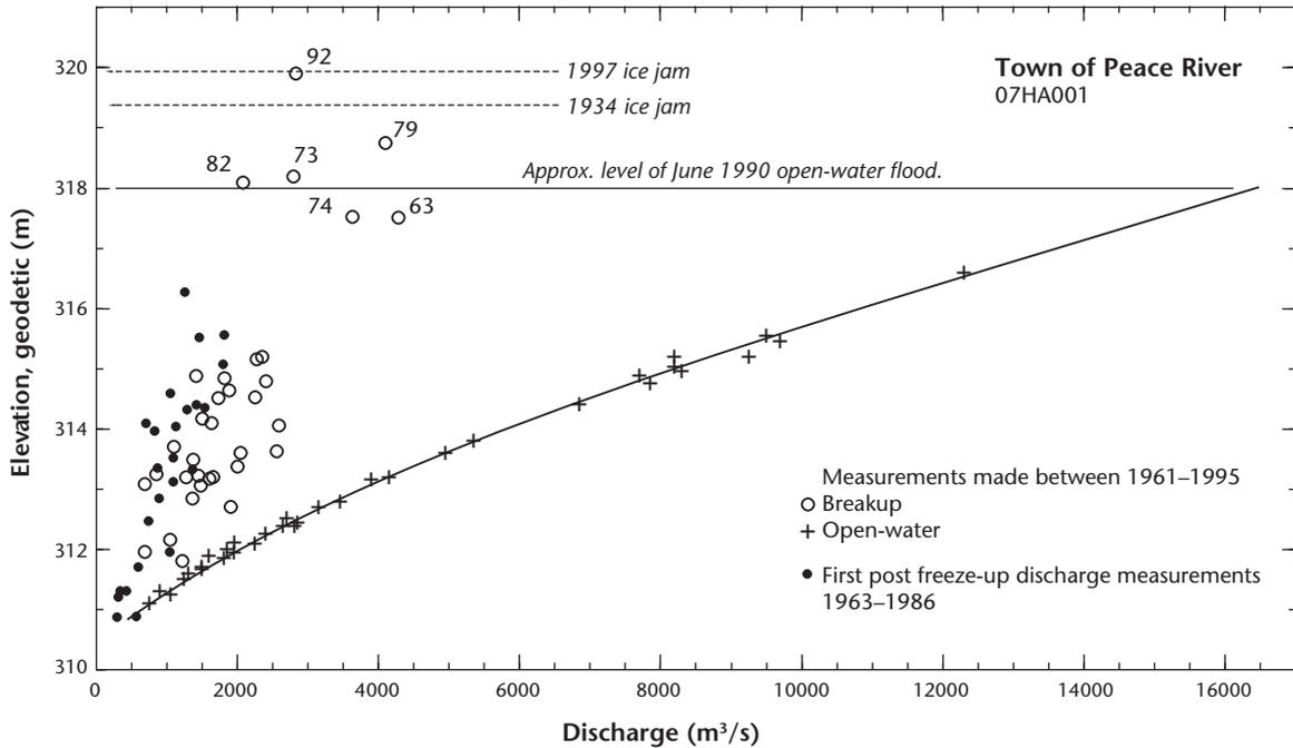
**Figure 6.3** Ice affected stages at TPR in comparison with open-water stages. The ice stages are treated as a single sequence before and after regulation. Freeze-up data from Andres (1995).
