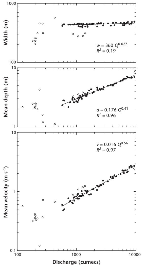
**Figure 5.5** WSC Stn. 07FD002, Peace River at Taylor: hydraulic geometry for open water, period 1944 to 1967, natural regime. Aberrant data (open symbols) are plotted but not included in the calculation of the best-fit function.  $R^2$  for width is poor because there is very little variation in width.
