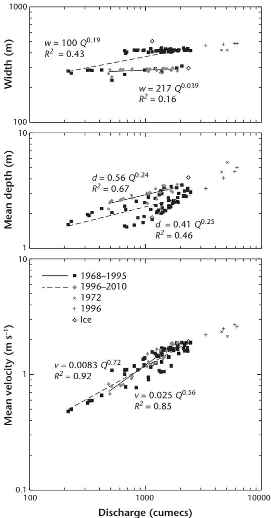
**Figure 5.6** WSC Stn. 07FD002, Peace River at Taylor: hydraulic geometry for open water, periods 1968 to 1995 and 1996 to 2010. Aberrant data are plotted but not included in the calculation of the best-fit functions. It is evident that the early period presents two geometries: see figure 5.7 for further analysis.
