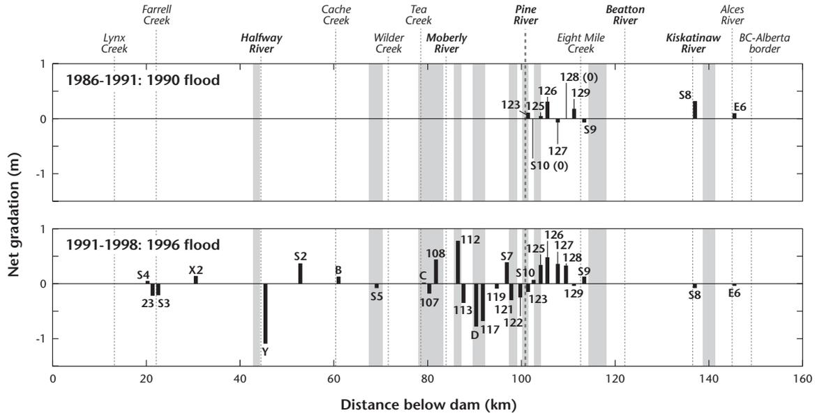
Figure 10.8 Pattern of erosion and sedimentation in the British Columbia reach of the river, plotted as net gradation at monumented cross-sections, resulting from the 1990 flood and 1996 release flow. Gray bars indicate significant sediment sources associated with landsliding.
