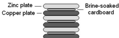
1786, Volta found that zinc and copper plates separated by cardboard soaked in brine produced a current. We have drawn three cells of a voltaic pile in Fig. 1.3.
