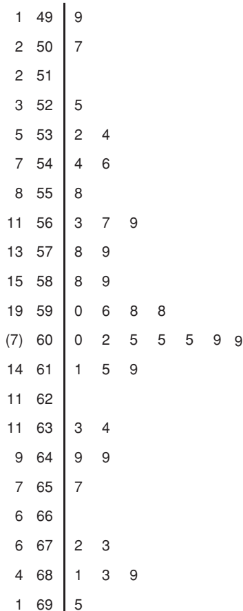
Fig. 1.3.1 Stem-and-leaf plot for compressive strengths of concrete in Table E.1.2; units for stem: 1 N/mm 2 ; units for leaves: 0.1 N/mm 2 .
