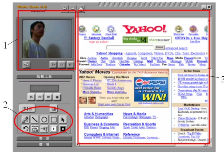
Fig. 3. Layout of Authoring Tool (1) Preview the video image of CCD, (2) authoring tool bar, and (3) browser and the area of course authoring
