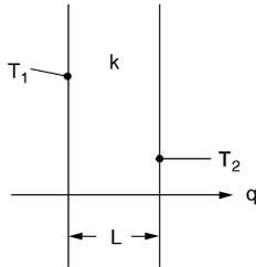
$$\dot{Q} = -kA(T_2 - T_1)/L, \text{ where}$$
