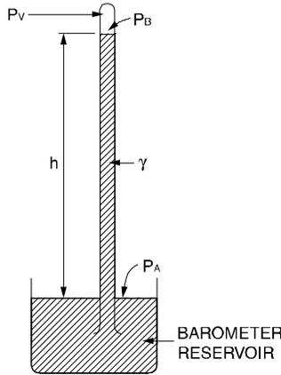
$p_v$  = vapor pressure of the barometer fluid
