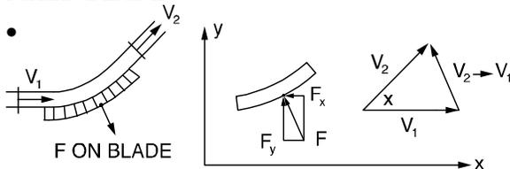
$$-F_x = Q\rho(V_2\cos\alpha - V_1)$$
