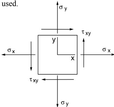
1. Tensile normal stress components are plotted on the horizontal axis and are considered positive. Compressive normal stress components are negative.
