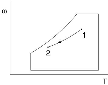
$$\dot{Q}_{out} = \dot{m}_a [(h_2 - h_1) + h_{f,3}(\omega_1 - \omega_2)]$$
