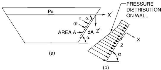
Forces on a submerged plane wall. (a) Submerged plane surface. (b) Pressure distribution.
