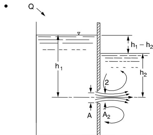
$$Q = A_2 V_2 = C_c C_v A \sqrt{2g(h_1 - h_2)} = CA \sqrt{2g(h_1 - h_2)}$$
