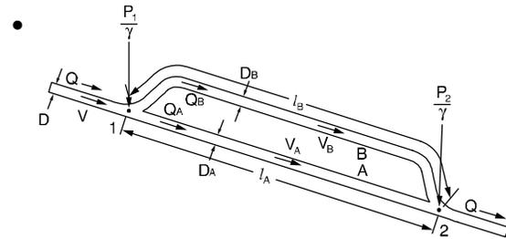
The same head loss occurs in each branch as in the combination of the two. The following equations may be solved simultaneously for  $V_A$  and  $V_B$ :
