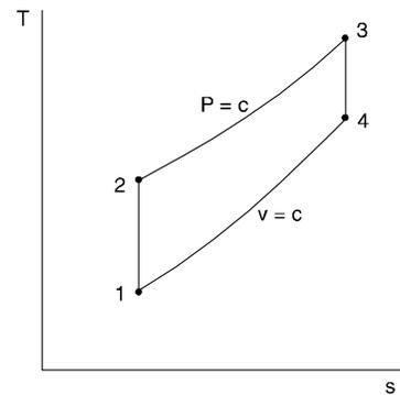
$$r = V_1/V_2$$
