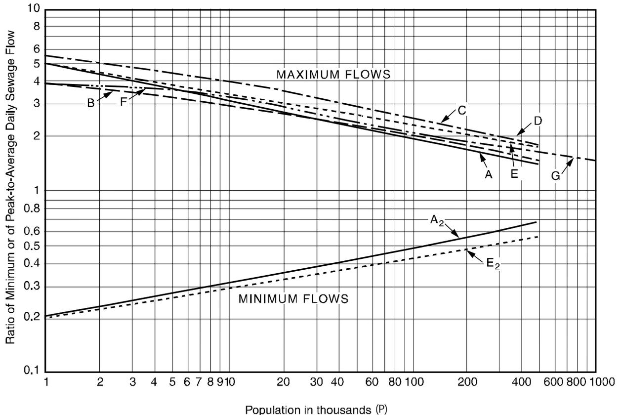
Curve A<sub>2</sub>:  $\frac{5}{P^{0.167}}$       Curve B:  $\frac{14}{4 + \sqrt{P}} + 1$       Curve G:  $\frac{18 + \sqrt{P}}{4 + \sqrt{P}}$
