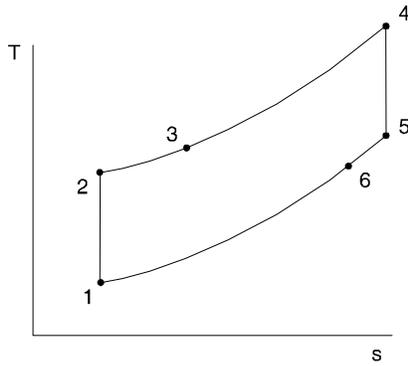
$$h_3 - h_2 = h_5 - h_6 \quad \text{or} \quad T_3 - T_2 = T_5 - T_6$$
