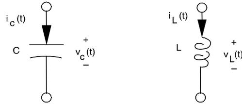
The charge  $q_C(t)$  and voltage  $v_C(t)$  relationship for a capacitor  $C$  in farads is
