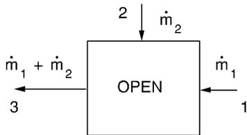
$$\dot{m}_1 h_1 + \dot{m}_2 h_2 = \dot{m}_3 (\dot{m}_1 + \dot{m}_2)$$
