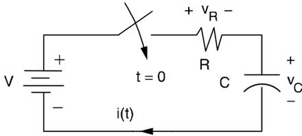
$$t \geq 0; v_C(t) = v_C(0)e^{-t/RC} + V(1 - e^{-t/RC})$$
