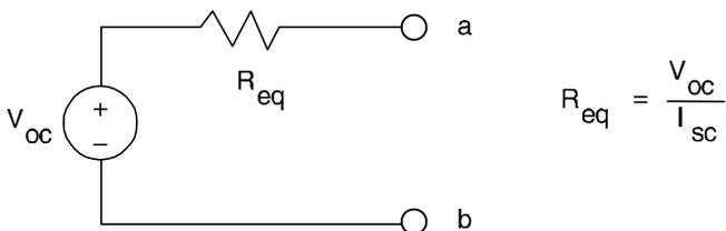
The open circuit voltage  $V_{oc}$  is  $V_a - V_b$ , and the short circuit current is  $I_{sc}$  from  $a$  to  $b$ .
