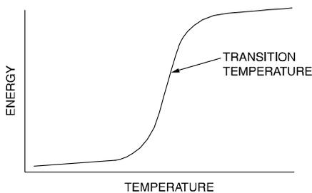
Impact tests determine the amount of energy required to cause failure in standardized test samples. The tests are repeated over a range of temperatures to determine the *transition temperature*.
