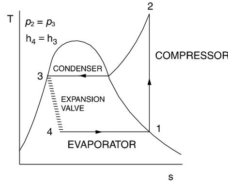
$COP_{ref} = \frac{h_1 - h_4}{h_2 - h_1}$        $COP_{HP} = \frac{h_2 - h_3}{h_2 - h_1}$
