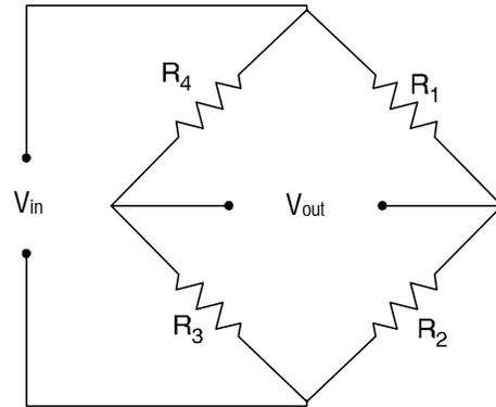
Half-bridge and full-bridge configurations use two or four variable resistors, respectively. A full-bridge strain gage circuit give a voltage output of
