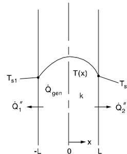
$$T(x) = \frac{\dot{Q}_{gen} L^2}{2k} \left( 1 - \frac{x^2}{L^2} \right) + \left( \frac{T_{s2} - T_{s1}}{2} \right) \left( \frac{x}{L} \right) + \left( \frac{T_{s1} + T_{s2}}{2} \right)$$
