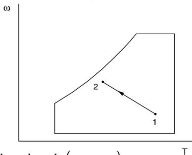
$$h_2 = h_1 + h_3(\omega_2 - \omega_1)$$
