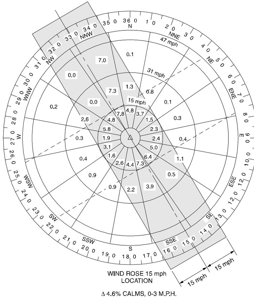
1. Cross-wind component of 12 mph maximum for aircraft of 12,500 lb or less weight and 15 mph maximum for aircraft weighing more than 12,500 lb.
