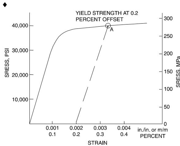
The slope of the linear portion of the curve equals the modulus of elasticity.
