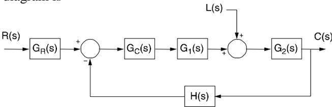
where  $G_R(s)$  describes an input processor,  $G_C(s)$  a controller or compensator,  $G_1(s)$  and  $G_2(s)$  represent a partitioned plant model, and  $H(s)$  a feedback function.  $C(s)$  represents the controlled variable,  $R(s)$  represents the setpoint, and  $L(s)$  represents a load disturbance.  $C(s)$  is related to  $R(s)$  and  $L(s)$  by
