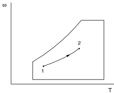
$$\dot{Q}_{in} = \dot{m}_a [(h_2 - h_1) + h_3(\omega_2 - \omega_1)]$$
