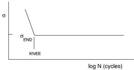
The *endurance stress* (*endurance limit* or *fatigue limit*) is the maximum stress which can be repeated indefinitely without causing failure. The *fatigue life* is the number of cycles required to cause failure for a given stress level.
