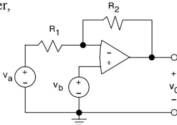
$$v_o = -\frac{R_2}{R_1}v_a + \left(1 + \frac{R_2}{R_1}\right)v_b$$
