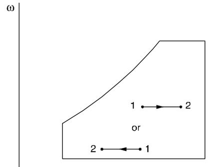
$$\dot{Q} = \dot{m}_a (h_2 - h_1) = \dot{m}_a C_{pm} (T_2 - T_1)$$
