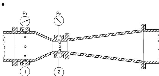
**Orifices** The cross-sectional area at the vena contracta  $A_2$  is characterized by a *coefficient of contraction*  $C_c$  and given by  $C_c A$ .
