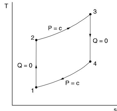
$$w_{12} = h_1 - h_2 = c_p (T_1 - T_2)$$
