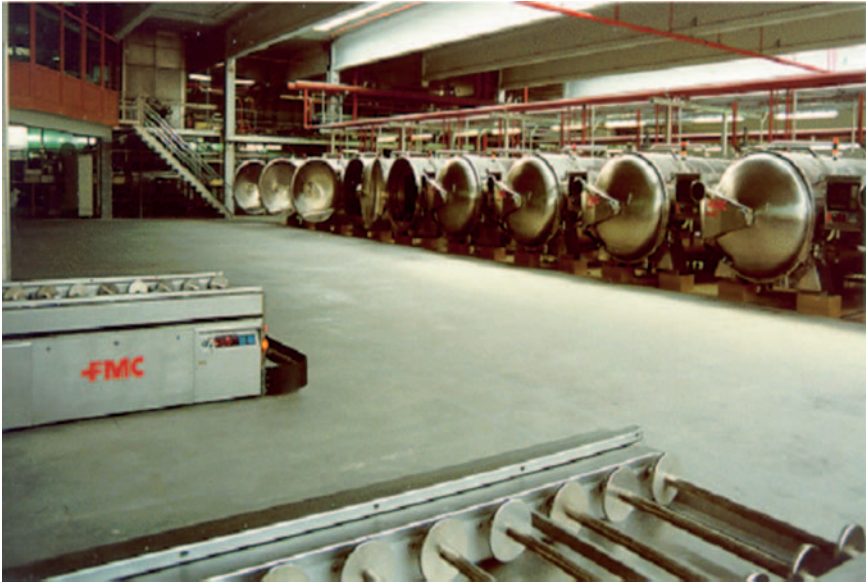
FIGURE 9.4. Automated batch retort system with use of automated guided vehicles in large Cook room operation (Courtesy, FMC Food Tech., Madera, CA).
