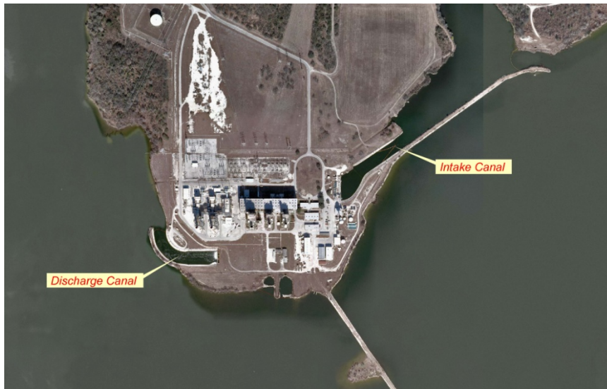
Figure 5-2. Braunig Lake Power Station. Intake at the northeast arm of the lake and discharge at the southern and western areas of the lake.
