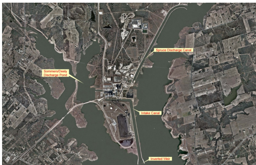
Figure 5-3. Calaveras Lake Power Station. The cooling water intake is from the rear of the 1.8-mile-long intake canal. Spruce plants discharge at the northeastern arm of the lake and Sommers/Deely plants discharge at the northwestern arm of the lake.
