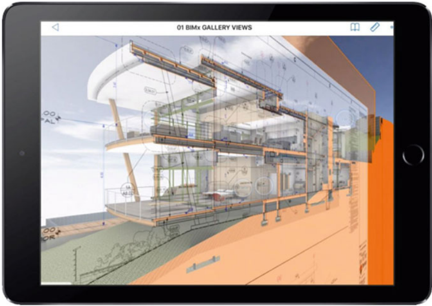
Fig. 20 Design shown in mobile apps (Graphisoft 2016). BIM is created with GRAPHISOFT ARCHICAD
