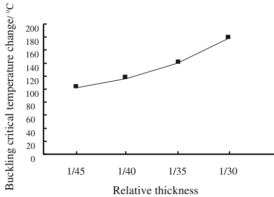
Fig. 4.6 The influence of the relative thickness on the critical buckling temperature variation
