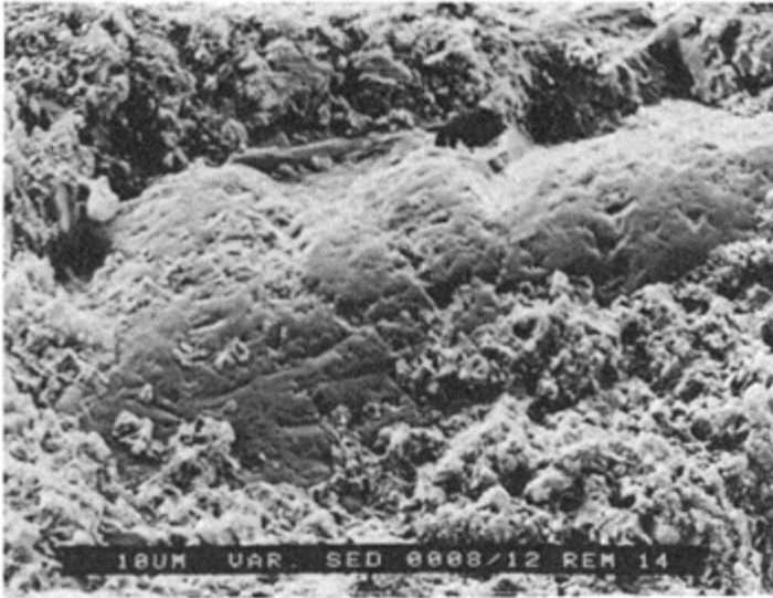
Fig. 8. Compact matrix in REM composite (640x).
