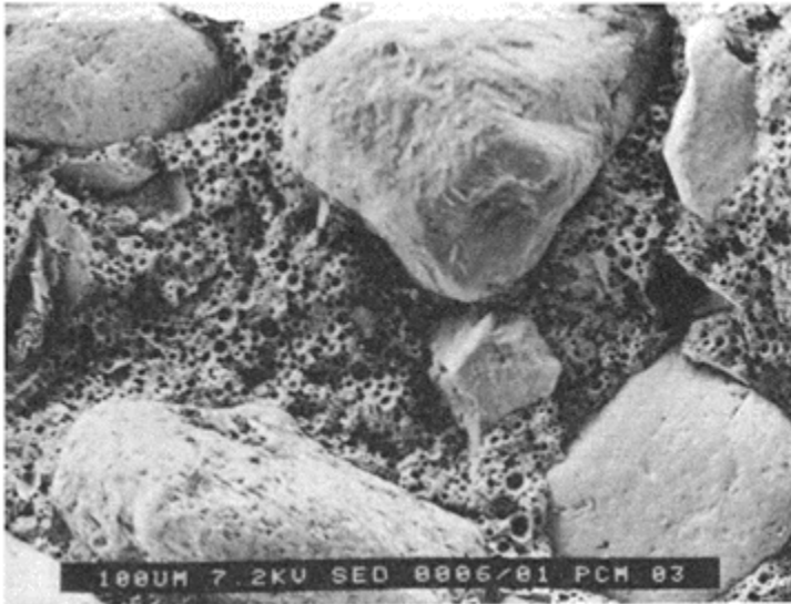
Fig. 4. General view of PCM microstructure (160x).
