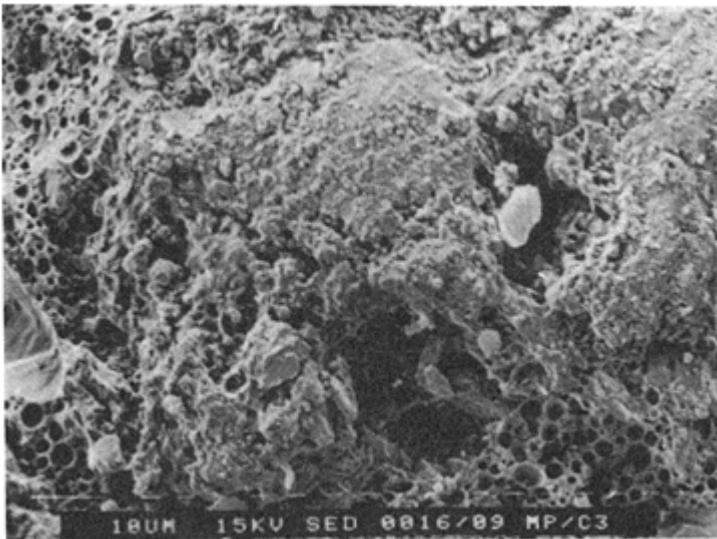
Fig. 5. Regions of PCM matrix presenting a more compact microstructure (320x).
