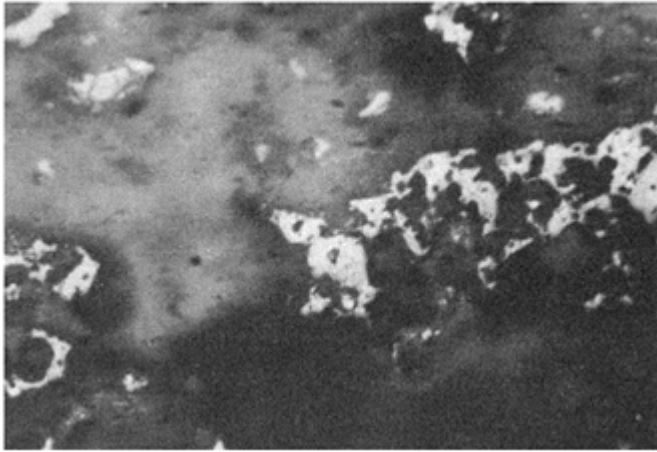
Fig. 4. The interface of the HCP and the ESG (above: HCP below: ESG)
