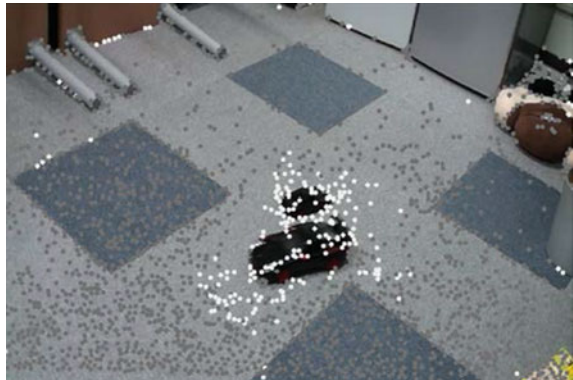
Fig. 3 Result of selecting process. The gray points are the feature points which are regarded as the points in the background and the white points are the selected feature points
