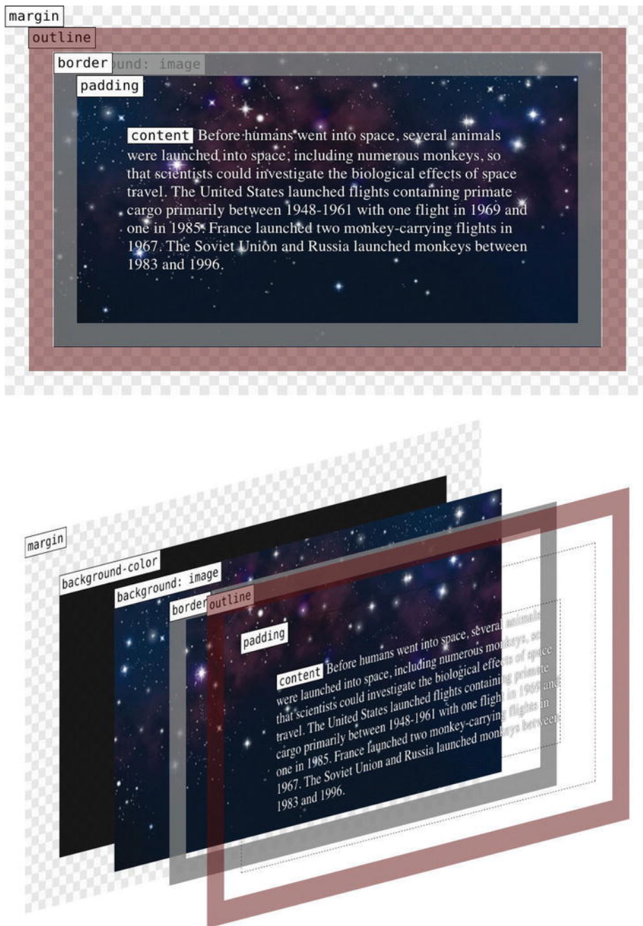
Figure 9-1. A CSS box (including outline), with an exploded view showing how the parts of a block-level box are stacked
