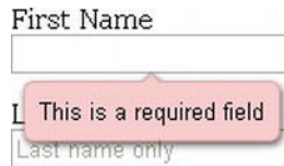
Figure 6-3. Form field with required attribute displaying a browser-generated error message in Opera
