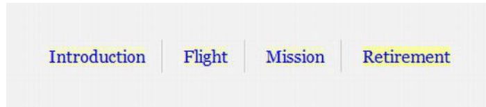
Figure 8-12. Navigation menu using :last-child to remove the right border from the last menu item
