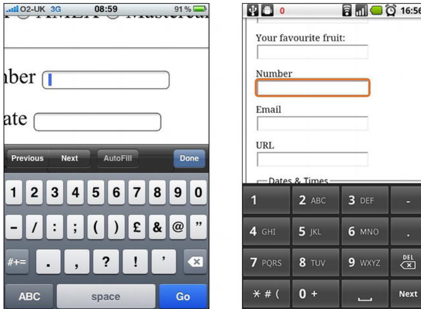
Figure 6-13. type=number on iPhone and Android HTC Desire (Android screenshot provided by Stuart Langridge)
