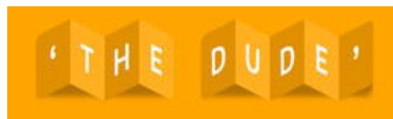
Figure 12-8. Using skew() for typographic effect, via Dave Rupert's Lettering.js
