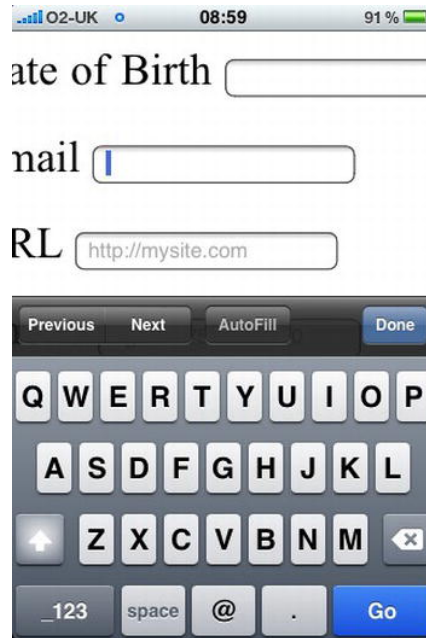
Figure 6-9. The iPhone displays a custom keyboard when using type="email" .
