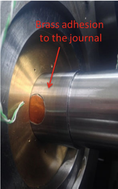
Fig. 8.18 Brass adhesion to the journal for the high detergent sample
