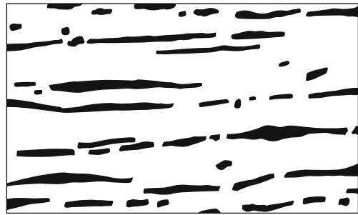
Figure 6.2 Microstructure of a typical wrought iron, with threads or strand of slag aligned in direction of rolling
