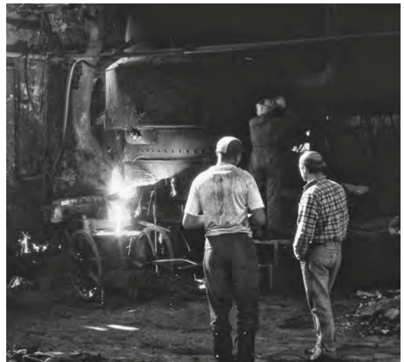
Figure 5.2 Tapping molten iron from the furnace prior to casting
