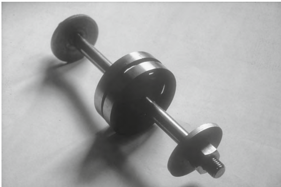
Figure 33.19 For the green oak structure at York Minster, shear plate connectors were used instead of split rings to accommodate the cross-grain drying shrinkage. © Arup
