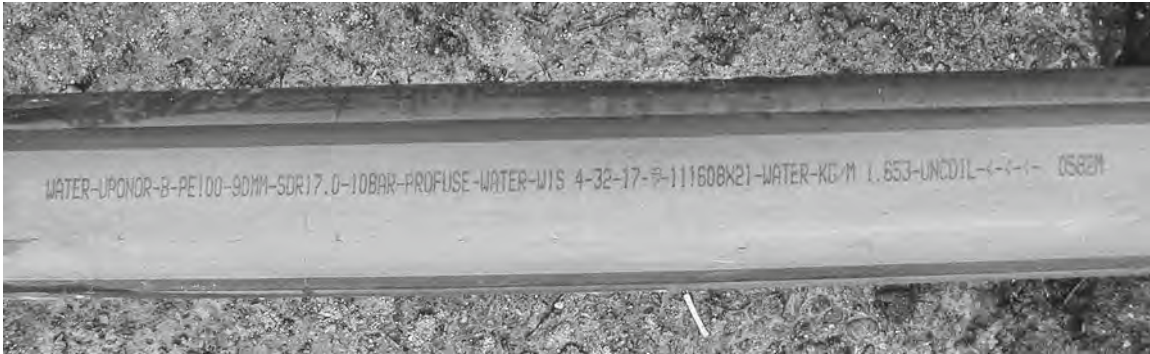
Figure 22.7 Typical markings on 90 mm PE100 water pipe
