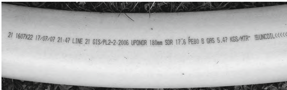
Figure 22.3 Typical markings on 75 and 180 mm PE80 gas pipe
