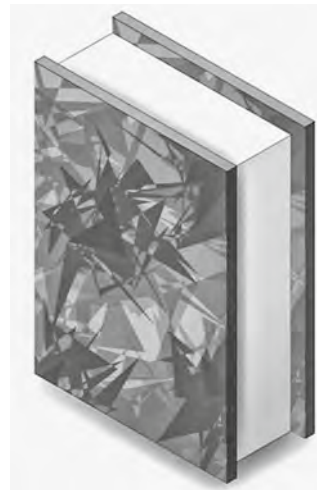
Figure 24.7 Cross-section of an SIP panel
