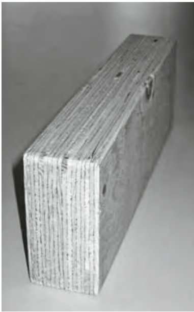
Figure 33.18 Laminated veneer lumber is made from 3 mm thick veneers. © Arup
