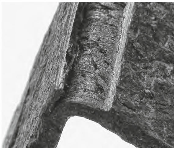
Figure 6.1 Typical fibrous surface of wrought iron plate exposed by cutting and then bending (courtesy of Thomas Swailes, University of Manchester)
