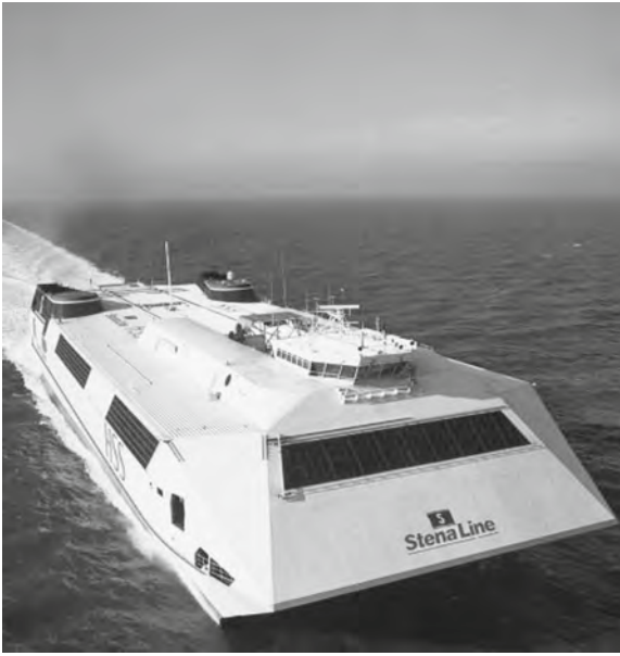
Figure 2.10 High-speed catamaran ferry with aluminium hull and superstructure
