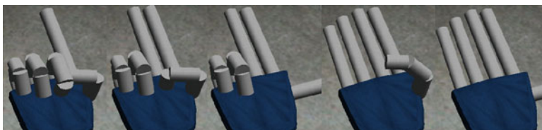
Fig. 9.2 Number representation with the right hand fingers of the iCub. From left to right: one, two, three, four and five
