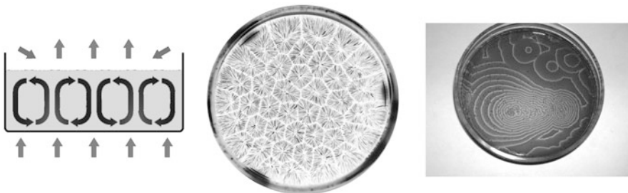
Fig. 4.1 Examples of self-organization in physics and chemistry. On the left a scheme of B enard’s convective cells, with the heated fluid directed upwards, and the coldest part directed downwards. In the middle a real image, with heated silicon oil, and the cells made visible thanks to graphite marker. On the right the B-Z reaction
