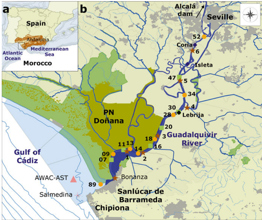
Fig. 8.1 Map of region, showing (a) Andalucía in Spain and (b) the Guadalquivir estuary with the indications of the instruments deployed and measurements made within the Guadalquivir monitoring network: Green squares correspond to water dynamics stations, orange dots to water quality stations, brown stars to tide gauges, pink triangle to AWAC-AST, pink star to Salmedina meteorological station, and diamonds to temporary quality stations
