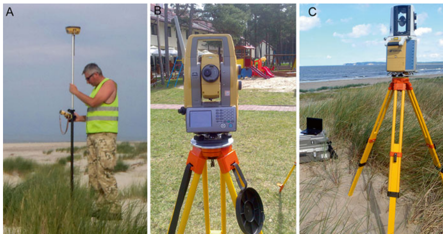
Fig. 14.8 The equipment used for dunes morphology surveying, (a) Real-Time Kinematic (RTK) GPS, (b) Total Station (TS), (c) Terrestrial Laser Scanner (TLS)
