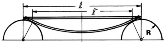
Fig. 2.2 A beam on circular supports of finite radius exhibiting periodic length variation during flexural vibration
