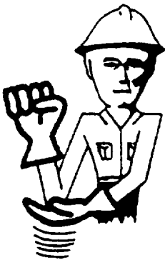
25 USE WHIP LINE. (AUXILIARY HOIST) TAP ELBOW WITH ONE HAND, THEN USE REGULAR SIGNALS.
