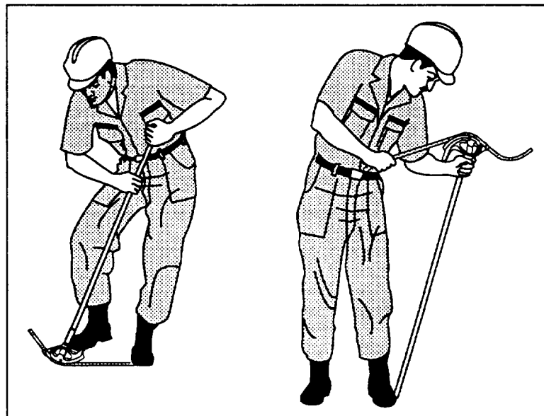
Figure 5-48.—Bending on the floor and in the air.
