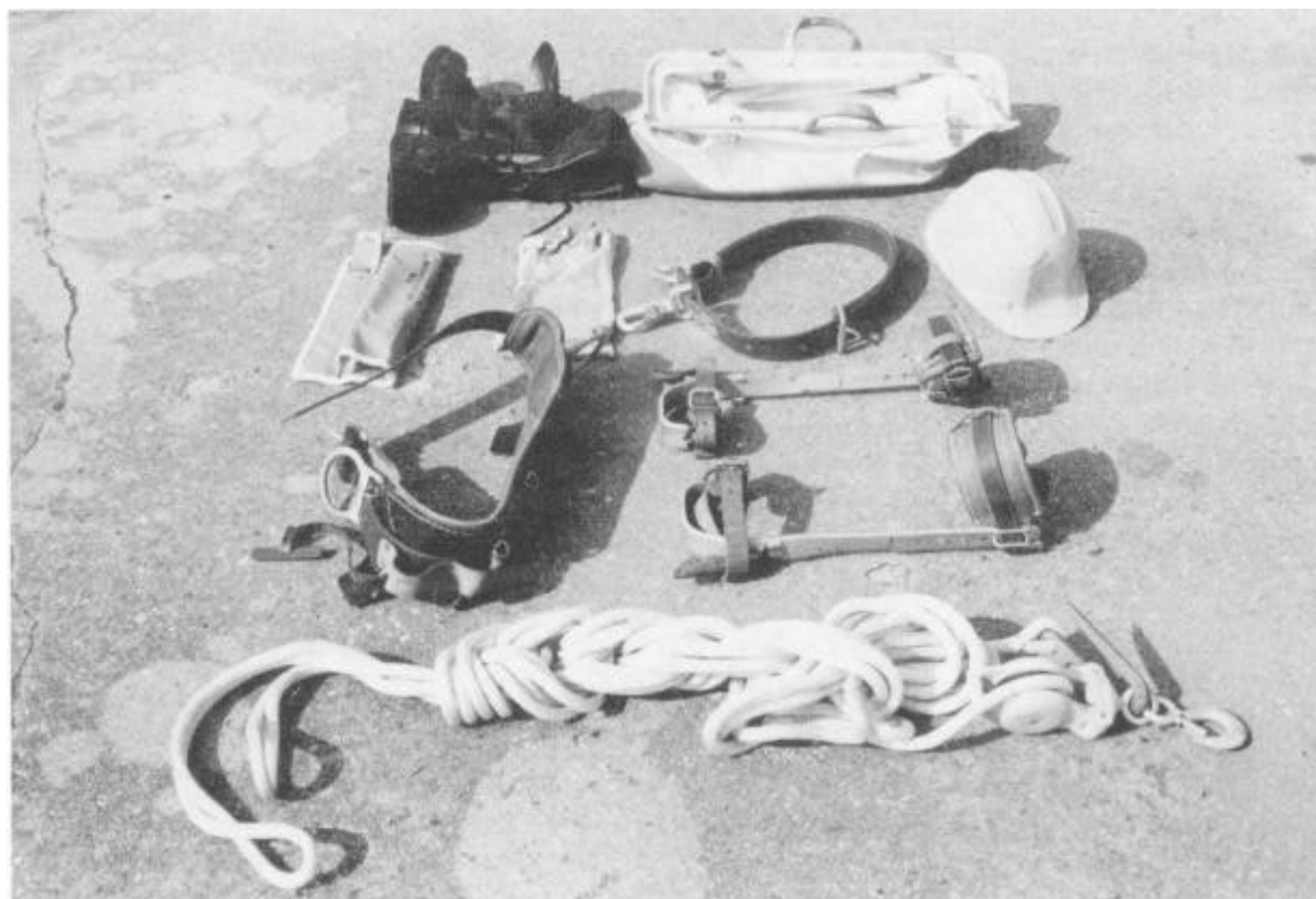
Figure 4-73.—Pole climbing equipment.
