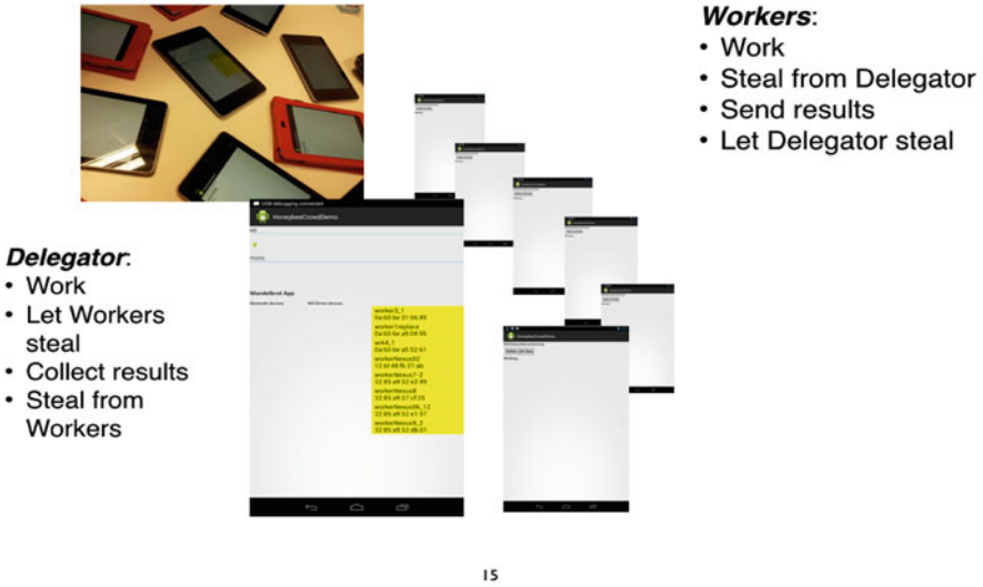
Fig. 2.1 Honeybee with workers and delegators. Note that in this implementation of Honeybee, the delegator steals from slow workers, and faster workers then steal from the delegator—we could also have faster workers steal from slower workers directly, though trading-off some delegator control
