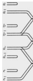
FIGURE 26 This shows how we can implement a disjunction of the CNF expression, such as “ a or b or not d or e ,” after pushing all the relevant variables out to the right. If one of the terms, say b , is true, then only the stubby path will be used there, and so, if any of a or not d or e is false, they may use the long path that leans toward b , and they will not cross each other. But if none of the terms is true, then there will not be enough room for all the falsehoods to be able to coexist without crossing each other.
