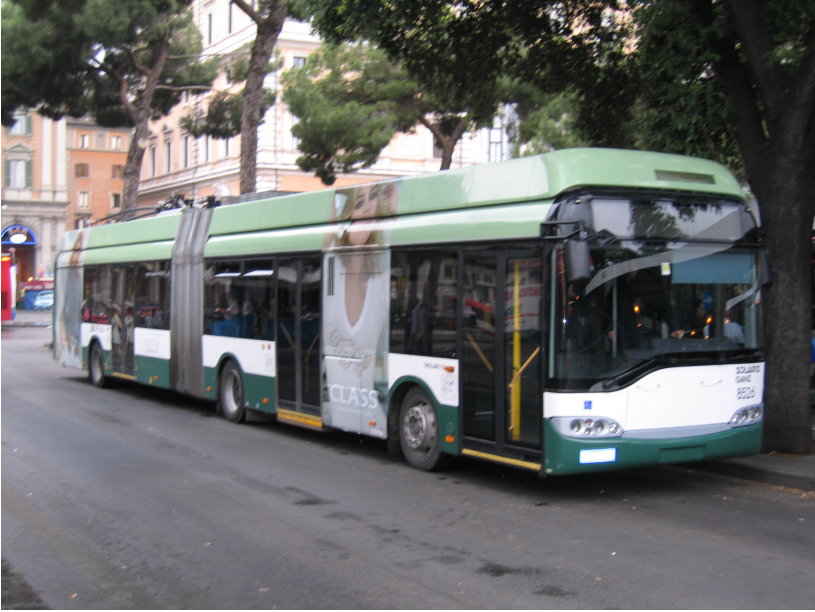
Fig. 11 New trolley bus capable of using power from overhead wires or battery, introduced in Rome to avoid air pollution
