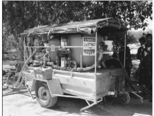
FIGURE 6-3 USAID Office of Foreign Disaster Assistance water purification unit that produced 78,000 liters of water per day for families affected by the January 2001 earthquake in India. (Source: Michael Ernst, USAID/OFDA.)
