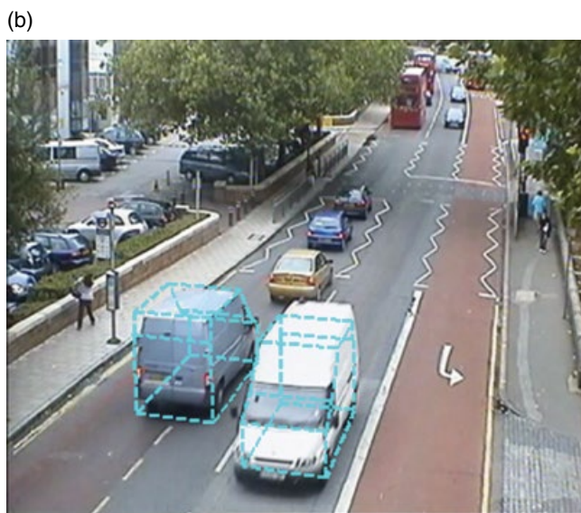
Figure 6.10 3D wireframe models with true size (a) and samples of their projections on the ground plane (b).
