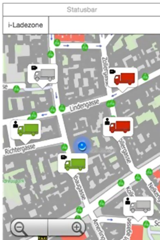
Figure 8.1 Example of a smart phone application developed for use by delivery trucks in the City of Vienna, Austria. Bright-colored truck icons indicate free loading zones, dark icons indicate occupied zones, and mid-gray color means “not in use.” Source: Adapted from Fluidtime , Vienna.
