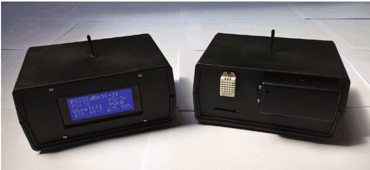
Fig. 2. Completely assembled WSN nodes: router and coordinator
