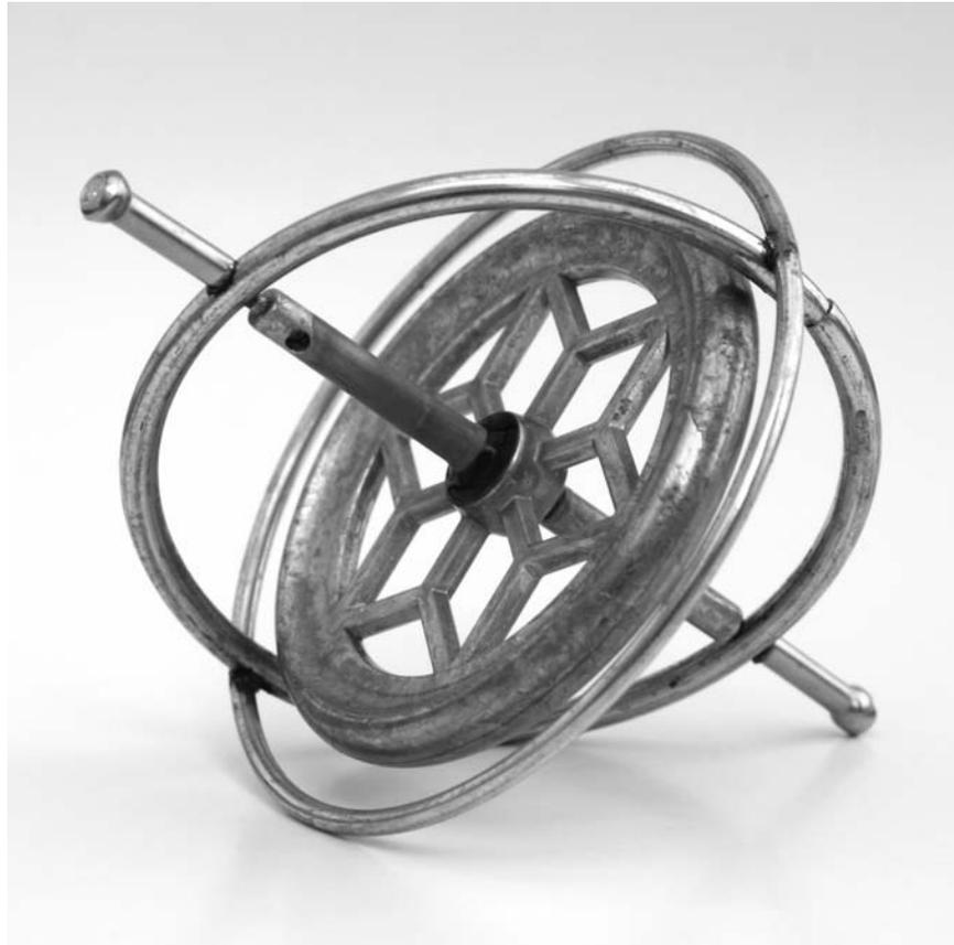
*A gyroscope is widely used in navigation instruments since the direction of its axis remains fixed. However, if a force is applied to one of the gimbals, the gyroscope will rotate about the axis that is parallel to the force. This motion, called precession, is analyzed in Probs. 19.80 and 19.81.*
