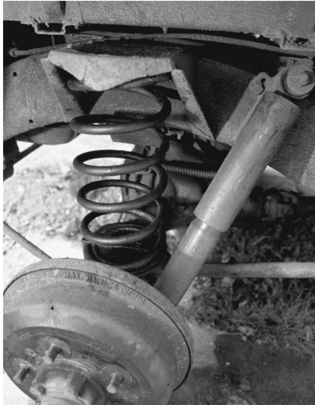
*An automobile suspension is an example of a damped mass-spring system, where the shock absorber provides the damping. Damped vibrations is one of the topics discussed in this chapter. (© Leslie Garland Picture Library/Alamy)*
