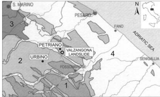
Fig. 1.1. Geological sketch of the Urbino area. 1) Limestones, marly limestones, marlstones and cherts (formations between Calcare Massiccio and Schlier, Lias – Miocene p.p.); 2) Arenites, pelites and evaporites (formations between Marnoso-Arenacea and Colombacci, Miocene p.p.); 3) Chaotic complex clays of the Marecchia Valley; 4) Clayey, sandy and gravelly deposits (Plio-Pleistocene). (From Antonini et al. 1993, modified).
