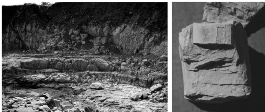
Fig. 2. Bedding of the Miocene blue clays at an outcrop of the Agrio River (left) and in a core taken below the dam and outside the landslide (right).
