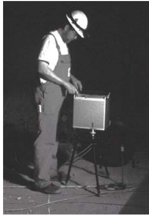
Fig. 4. Micro-gravity surveys for cavity detection along the Irlahüll tunnel.
