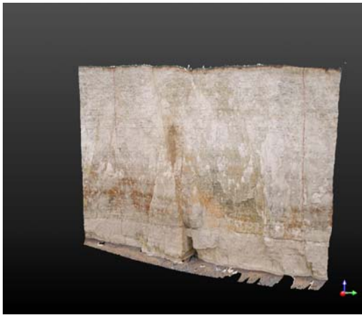
Fig. 7. 3D digital rendering of a point cloud of a limestone cliff along the westcoast of France made using a Riegler LMS-Z420i system. Each individual point in the “cloud” is coloured using a high-resolution digital camera. (Data: Riegler).
