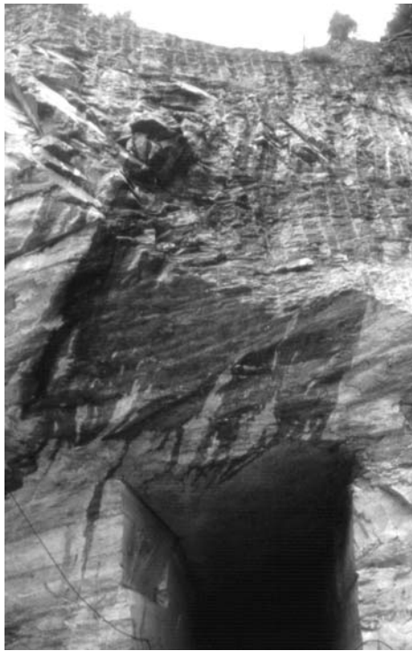
Fig. 2. The thick rock cap above the exploitable bank where the underground experimentation has been driven.
