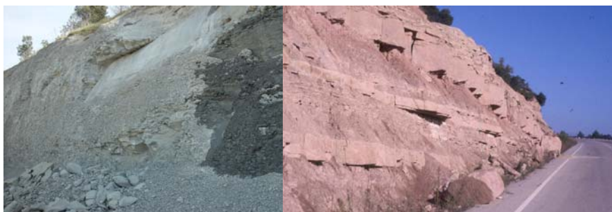
Fig. 1. (a -left) Breakdown of marls, with fragments accumulation at the slope foot and generation of listric joints responsible for the failure. Cut slope near Vic (Barcelona); (b – right) Rock falls produced by overhanging and subsequent toppling of sandstone layers in a cut slope near Solsona (Lleida). The process is accelerated by rapid disintegration of the underlying mudstones.
