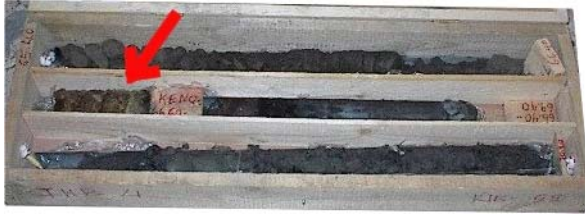
Fig. 8. Part of timber support encountered in borehole THP-4.
