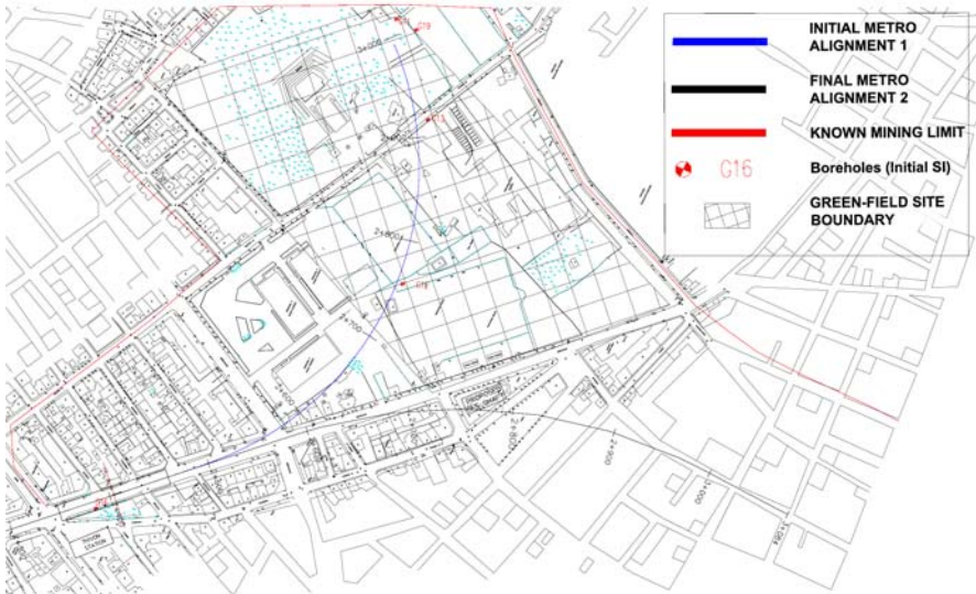
Fig. 2. Plan view of Metro Alignment, location of initial investigation boreholes (Marinos P., 2000).
