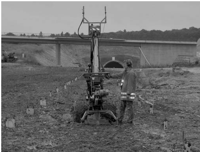
Fig. 3. Seismic measurements using a weight drop for generating elastic waves and the SUMMIT data acquisition system.
