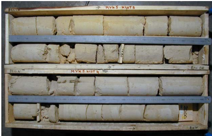
Fig. 6. Sample (core) box showing limestone of Emael. Length core box equals approximately 1 m.
