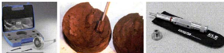
Fig. 2.4. Vane shear test and pocket penetrometer.
